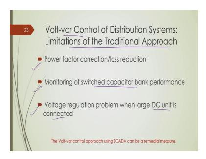
Now, these are the limitations of traditional approaches for volt-var control. What do you mean by traditional approaches? Traditional approaches are deployment of capacitor bank and traditional approaches are also make use of on-load tap changer, ok. They have some limitations. So, these limitations are: they have certain capability of loss reduction and also they have some switching problem, ok.
