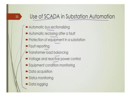
Now, use of SCADA in substation automation: so, as I said SCADA is a backbone of automated distribution system operation and it is useful for substation automation as well. So, we can do many things by using the SCADA system which includes automated bus sectionalizing, automatic reclosing after a fault, fault reporting, protection, transformer load balancing, voltage and reactive power control etc., ok.
