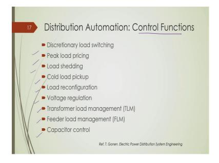
So, these are the control functionalities of distribution automation, load switching, peak load pricing, load shedding; automated load shedding of course, this cold load pickup, reconfiguration, voltage regulation, transformer load management, feeder load management, capacitor control. Those things, at this point we know many things.
