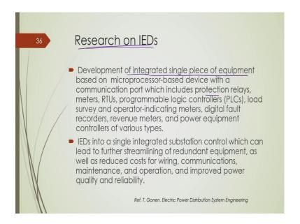
As I said, there are many research papers reported last few years on the development of IEDs which are basically aimed at development of integrated single piece of equipment. Of course, it is microprocessor based device in order to have various you know properties which include protection, which include metering, which include load management etcetera, ok.
