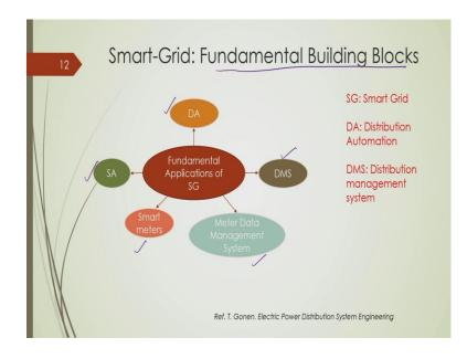
And also I discussed the different fundamental building blocks of a smart grid which include different building blocks, for example, distribution automation, substation automation, distribution management system or DMS, smart metering system, and meter data management system. So, these building blocks will try to describe in more detail in this lecture, ok.
