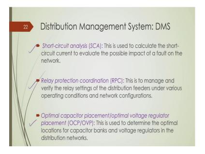
Also, it has short circuit analysis capability, this relay protection coordination system and optimal capacitor placement, ok which I was also talking talked about in module 5, ok.
