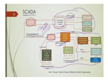
So, this is a typical, you know, schematic diagram of a SCADA system, ok. SCADA as I said, it is a backbone of automation of a distribution system, ok. Now, in this SCADA system, this part is the this part is your master station. This is the master station. And this part is basically remote station. And in between them, there are few kilometers distance. So, they are located few kilometers distant, few kilometers distant, ok.
