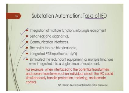
And what are the tasks of IEDs, we have in a substation automation process? There are multiple tasks which include integration of multiple functions into a single equipment, self check and diagnostic or self-healing process, this communication interface ability to store historical data and there are many others, ok.
