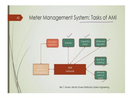
And these are the typical tasks of automated metering infrastructure network. It needs to be connected with operation of the switches, capacitor banks, distributed regulators, real time metering and alternating point of supply, ok.
