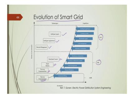
So, this is a figure which gives you again similar kind of advancement starting from this one-way communication to two-way communication deployment of smart sensor and distributed control. This is possible by using AMI, automated metering infrastructure. And next step ahead is basically smart grid which needs network management intelligent application and intelligent agents, ok. And of course, their functionalities will also increase, so as the investment and return on the investment, ok.
