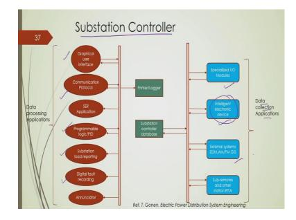
So, this is a typical, you know, schematic part substation controller. There are many things connected with this which include graphical user interface, communication protocol, substation load reporting, programmable logic, digital fault recording, etc. And also, there are some data collection applications, for example, input output modules, intelligent electronic device, IED I was talking about, and many others.
