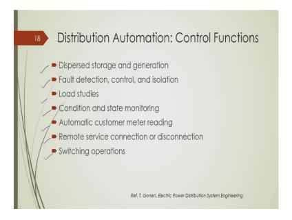
And also, this presence of storage, fault, automated fault detection, load studies, condition and state monitoring, automated meter reading, remote service connection and switching, these are the some of the functionalities of distribution automation, ok.
