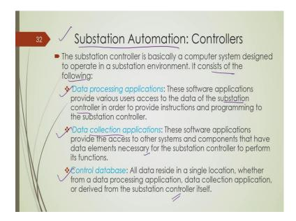
Now, next building block for automated distribution system operation is called substation automations, ok. Substation automation consists of the following attributes, one is called data processing application, one is called data collection application, another is called control database.
