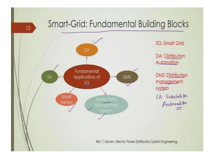
So, these are the building blocks of a typical smart grid and I will be discussing all these blocks in one by one in detail in more detail. So, this DA stands for Distribution Automation ok, this DMS stands Distribution Management System; then meter data or automated metering infrastructure which I will be discussing, smart meters and this meter data management system those I will be discussing.
