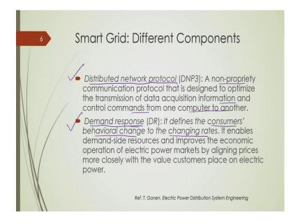
Now, since we are talking about this communication system, so, we will be having some protocol, communication protocol. And, there is a Distributed Network Protocol: DNP which is definition is non-proprietary communication protocol that is designed to optimize the transmission of data acquisition information and control commands from one computer to another computer.
