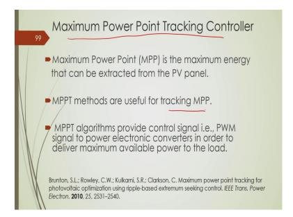
I am just keeping on, this is a typical output current characteristics of PV cell, and this is the point which I was trying to mention one, that is called maximum power point tracking, which means that where we intend to operate any solar PV conversion system to its maximum power point correspond to this maximum value of power from here, from which we get. And there are many approaches to track this maximum power point ok.
