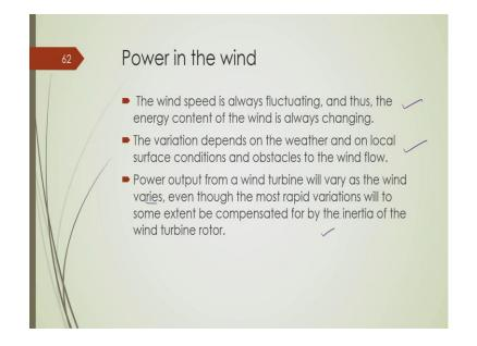
So, wind turbine is of intermittent nature and it depends upon weather; and power output of a wind turbine will vary as the wind varies ok, even though most of the rapid variation will be some extent compensated by the energy of the wind turbine rotor.
