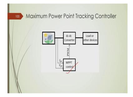
In fact, this is an area of research and people do use many types of MPPT control, MPPT stands for Maximum Power Point Tracking control so that we can always operate the solar PV system to its maximum power point ok.
