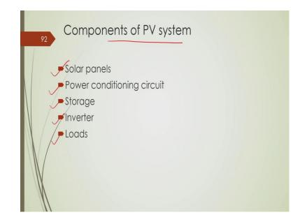
So, with a typical example that would be clear. But in typical photovoltaic system, we also have different other system along with the solar panel. One is called power conditioning circuit, storage, storage is required particularly if it is operated in isolated condition, without this connection with the grid, also inverters to convert this DC to AC and loads which is of course there.
