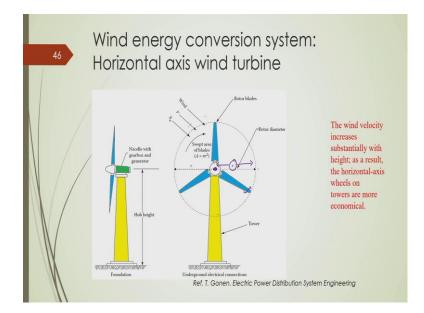
So, it is the, I can show you I can go back and show you. It is the area under this circle, suppose this typical 3 blade wind turbine, say, this is the center of the turbine or the swept of the turbine and suppose this is the radius ok r, which is almost equal to the length of the blade ok, length of a typical blade. So, if this is r, this is radius which is r and it forms a circular area then this area is called swept area, we discussed in the last lecture ok.
