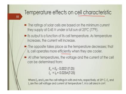
So, as I said, a typical voltage in a solar cell depends upon the temperature as well as solar irradiation. So, in fact, solar cell generation will vary with these different seasons, in winter and in summer there will be different ambient temperature, accordingly the solar generation would also vary and also it depends upon the solar irradiation ok.
