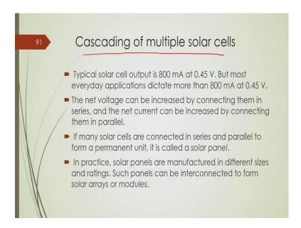
Now, as we know that we need to cascade because one typical solar cell will give you only a fractional voltage lesser than once. But in order to use them for typical applications in different, for a different point of a network or a different, for different customers we need to have a cascaded form of the solar cell and that cascading is done in order to achieve a desired value of voltage and in order to achieve desired amount of power ok.
