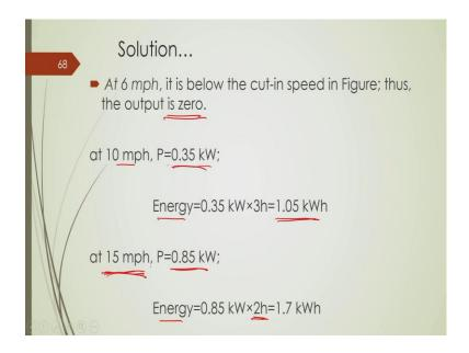
So, you can find out in different operating condition, one is 6 mile per hour, 15 mile per hour, 10 mile per hour and 20 mile per hour. So, corresponding to these values you can find out. So, this is 6 mile per hour and then next is 10 mile per hour, then next is 15 mile per hour and another is 20 mile per hour. So, corresponding to this, you can find out that how much power is available in the wind ok.
