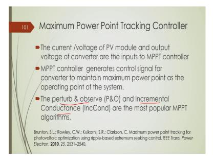
There are some typical MPPT techniques available, one is called perturb and observe technique, another is called incremental conductance technique, there are many other techniques as well which typically, which are typically employed to operate the solar cell to it maximum power ok.
