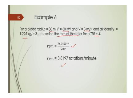
So, these are some examples where you can see that blade radius is given, power output is given, velocity is given, air density is given, TSR is given. So, you have to (Refer Time: 28:47) determine the rpm of the rotor. And similar way, this tip speed ratio expression that you have seen, it is also, you can find out with this TSR is nothing but tangential speed which is omega r divided by this wind speed. So, you can find out.
