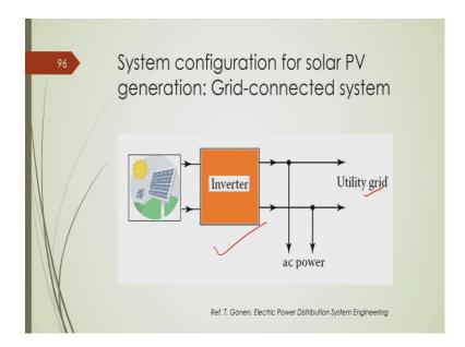
And grid connected mode does not need any storage, it can be directly connected to the grid and maximum and mismatch power that is surplus power or deficit power would be sent to the grid or to be imported to from the grid.
