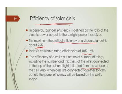
Now, the efficiency of the solar cell is again the matter of interest to us, but we know that maximum theoretical efficiency of a solar cell is only around 20 to 25 percent ok. So, this power density of this solar cell is very poor ok, and this is the maximum theoretical value, but actual efficiency is only 10 to 15 percent ok.
