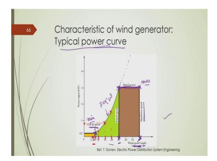
So, let me show you this typical power curve, this is called power curve which means that power out input versus this wind speed, power input versus this wind speed. Now, this gives you that there are some, there are some operating points, one is this operating point which is called cutting speed ok. So, this is the minimum speed at which this wind turbine would operate. So, below this cutting speed we cannot operate a wind turbine ok.
