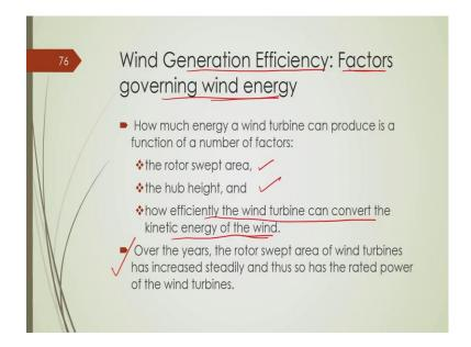
Now, that is the most important point that I am trying to make that, this wind power is not the power output of a wind turbine. That is basically power available in the wind and we have some factors to be multiplied in order to find out the output of the wind turbine. So, whatever this expression you have seen, that P is equal to half rho a V cube, that expression gives you the power availability in the wind, but that does not give you the power output of the interval ok.
