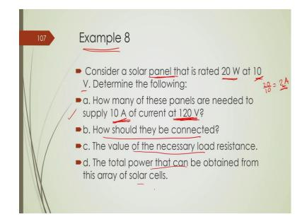
Now, here we have some examples, numerical examples, first numerical example is, suppose, we have a solar panel which consists of many solar cells which are rated of 20 watt and can produce 10 volt ok. Now, you have to decide that how many such solar panel we can make in series parallel combination in order to determine, in order to supply 120 volt at 10 ampere ok.
