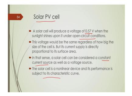
So, in a in a typical photovoltaic solar cell, it produces only a DC voltage of 0.57 ok, and it is open circuit voltage, I will show you the typical voltage and current characteristics for a typical solar cell. In a typical solar cell, it can be considered as a constant current source ok. And it is a non-linear device, its performance depends upon the characteristic curve.
