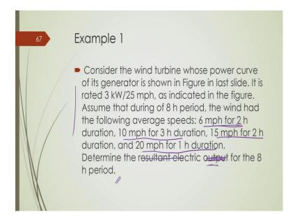
Now, we have an example; so this example is very simple and it is based upon this figure shown over this slide, that we have different wind speeds in different duration of a day ok. So, for 2 hours the wind speed is 6 mile per hour, for 3 hours wind speed is 10 mile per hour and for 2 hours wind speed is 15 mile per hour and for 1 hour the wind speed is 20 mile per hour.
