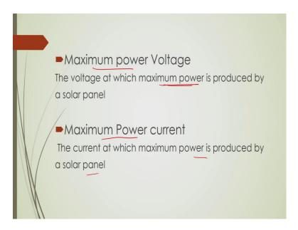
Now, there is another definition called maximum power voltage, which corresponds to the maximum power produced by a solar panel. So, voltage and current corresponding to maximum power, it is a matter of interest and maximum power current at which maximum power is produced by a current at which maximum power is produced by a solar panel. So, maximum power voltage, maximum power current corresponds to the maximum power produced by a solar panel.
