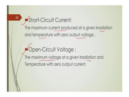
So, before I show you this characteristics curve, we have different definitions that one needs to know. One is called short circuit current: the short circuit current is maximum current produced at a given irradiation and temperature with 0 output voltage. Short circuit means output voltage is 0 and it gives you maximum current. And open circuit
