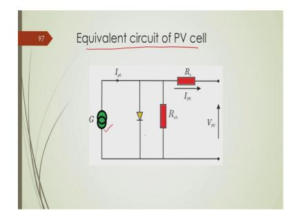
This is the equivalence electrical circuit form of this PV cell, it gives a current source, some diode and some resistances. This is required to devise the control of the solar PV and in order to do the further research on solar sensor.
