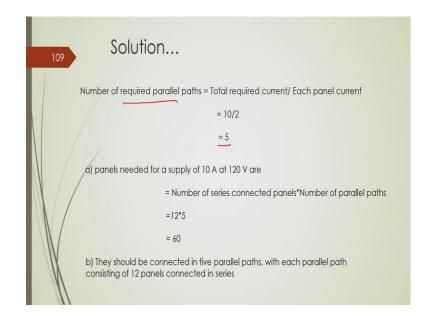
So, number of panels to be series is 12 and number of parallel paths that we require 5. So, it will be at 12 multiplied by 5; 12 solar panels would be connected in series and such kind of unit, 5 such kind of unit needs to be connected to parallel in order to have this required voltage and power ok. Now, another question is how they should be connected? So, you already determined that and the value of the necessary load resistance and total power that can be obtained from the solar cell.
