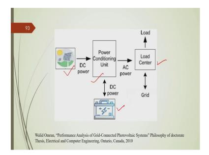
So, this is a typical, you know solar PV conversion system as a whole, which includes this solar cell, which includes power conditioning unit which includes this, you know inside power conditioning unit to converter is a, inverter is there in order to connect with the load ok. Also, this storage is an optional option which is required sometimes to store the surplus energy and to discharge when there is deficit energy ok.
