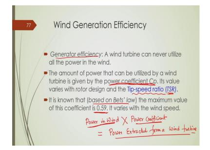
So, those things are there, but apart from that we have one another different parameter, one is called efficiency of the generator and also efficiency of all stakeholder, who are there in this wind energy conversion system. One is called efficiency of the gear box, which is used to change this rotation, rotational speed of the wind turbine to the speed of the rotational speed of this wind turbine blade to the speed of the generator, at which we would like to generate.
