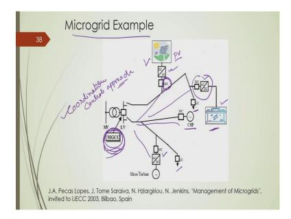
So, this is a typical microgrid. This is itself a complete microgrid where we have here central controller and there micro controller which exist in different sources which is called as micro source controller in different sources. For example, here we have photovoltaic P source. So, it is connected with the conventional microgrid with this
