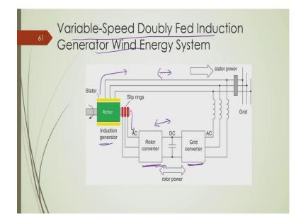
So, the schematic of this is shown over here. So, this is the schematic of doubly fed induction generator which is having two way of power flow. One is connecting with the stator another is through this slip ring through rotor ok. So, here we have two converters
