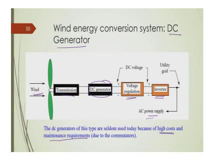
This is a typical DC generator which is not used nowadays, but it was used long time ago when this base operation of this wind mill started with. So, here we have you know this is the power available in the wind; it is extracted and it is being transmitted to this DC generator which converts this to DC voltage.
