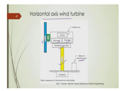
Now, there are many building blocks in a typical horizontal axis wind turbine which includes this rotor of course. Then, this is hub; there are some controllers, controller inbuilt available there, some drive train main generator. Then main frame or yaw system then, this is founded over a tower and we have some electrical system in order to extract power or in order to bring power from that particular wind turbine.
