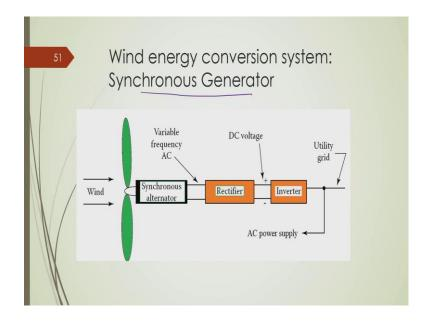
This is a synchronous generator; generally permanent magnet synchronous generator is used and this is the rectifier and inverter unit in order to supply which connects this to the grid with proper synchronized voltage and frequency.
