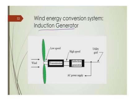
So, this is a typical induction generator type of wind energies conversion system which is similar to this synchronous generator. We have this arrangement same and then we have this induction generator which connects it to the AC power system ok.
