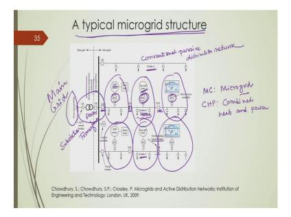
So, this is here a typical microgrid structure is shown in this figure; look at this figure very carefully. So, here we have this main grid, this is our main grid ok. So, we have a power transformer here, this is power transformer and then this is basically substation. This is where we have this power transformer and the bus bar arrangement to feed the load. And here we have 3 feeders; one is feeder A, another is feeder B, another is feeder C.
