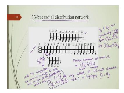
And we have simulated this by 33-node distribution network, as this network is known to you. So, what we did actually; starting from this bus number 2 to bus number 33, I exercise by connecting one DG unit at a time. For example, at one instant of time, I connect a DG unit at this bus number 2 or node number 2, ok.
