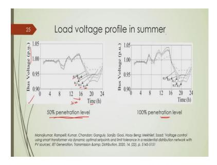
So, what we can see here with the 50 percent penetration level, these are the voltage profiles individual voltage profile; these are the time and these are the voltage profile in per unit and these are the voltage profiles in different you know loading points RL 1, RL 2, RL 3.
