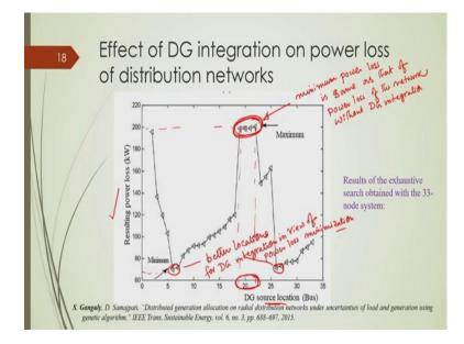
So, different locations, we get different minimum power loss and these minimum power losses are plotted, minimum power loss with respect to different locations of different nodes. So, you can see there are some locations, we get minimum power loss as same as the actual power loss without DG integration.
