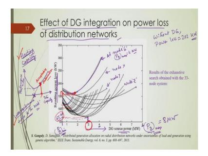
So, in order to understand this DG integration or in order to understand the effect or impact of DG integration on these different operational features of power distribution networks, what we did, we first determine these power losses with respect to this, with respect to different size of the DG, ok.
