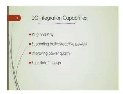
So, DG integration capabilities is a type of plug and play, it supports active and it can support reactive power as well; it can improve power quality, it can have fault ride through capability. (Refer Slide Time: 37:38)
