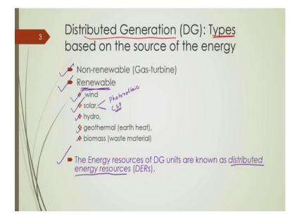
Now, as I said, where although types are not significant or relevant while defining the distributed generation; but we have different types of distributed generation units or different types of DG units. Which can be categorized as these 2 group; one is called non-renewable type, which are conventional type of gas turbine units having smaller capacity, but directly integrated to the distribution networks or may be renewable type of distributed generation units.
