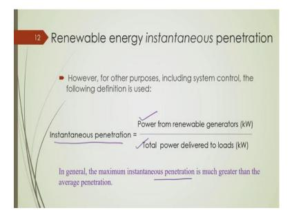
And instantaneous penetration is basically that it is a time varying quantity. So, it is ratio of power generated by a renewable generating unit to the total power delivered to the load, ok.
