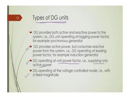
Now, we can also define different DG units on the basis of their operation or their ability to provide reactive power. So, one type of DG unit, in fact as I should say at this point that, the conventional power stations in India or even in other countries, the conventional generation comes from the fossil fuel based power plant, where we have synchronous generator, where we have synchronous generator.
