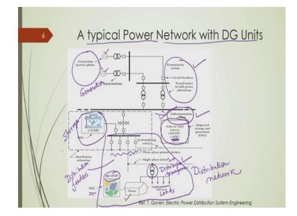
This is a typical illustration of distribution network with DG units; in fact this part is basically distribution networks. So, this is our distribution network, this part is subtransmission network as it is mentioned and this part is transmission system and this part is generation system.
