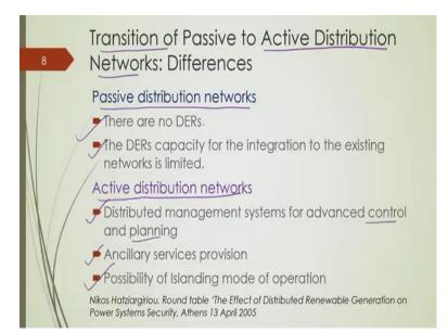
Now, with the integration of DG, with the integration of distributed generation, our distribution networks are slowly in the process of transition, in the process of transition to active distribution networks from the usual passive distribution networks.
