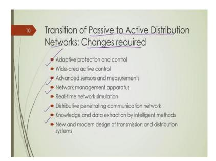
So, we need some changes; we need some changes, in order to have this smooth transition from passive to active distribution networks. Now, what are the changes we require? As I said protection system should be completely redesigned and accordingly new control strategy is to be devised, ok. So, many sensors and measurements should be required, so that the whole network state would be fully visible.
