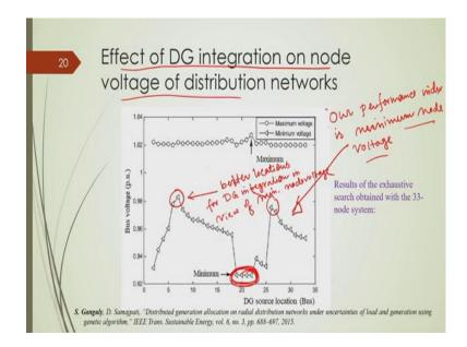
Similarly, we can also check the effect of DG integration on node voltage, ok. You can see here we consider minimum node voltage as the performance index. So, here our performance index is minimum node voltage, ok. So, this is the performance index. And you can see you know there are some locations, as well, where minimum node voltage was similar as that of the case without DG integration ok, but there are some points here and here you will get.
