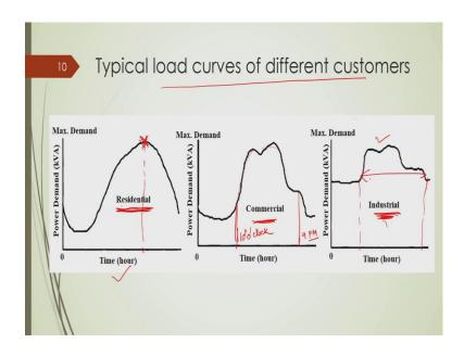
Now, this slide is to give an illustration that how different the load demand characteristics are for different types of customer. This is the typical load demand characteristics for not residential customer, but I can say that a distribution network which is serving in residential area ok.
