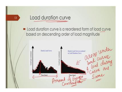
Now, again as I said in my previous slide that load duration curve is a reordered form of load curve. So, in load curve we can actually find out that when this load demand happens that for example, this the peak demand happens at during this particular of time.
