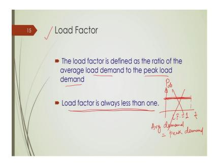
Now, we will be talking about certain factors or indices in order to model this load; one is called load factor ok. What do you mean by load factor? Load factor is basically defined as the ratio of the average load demand to the peak load demand ok.
