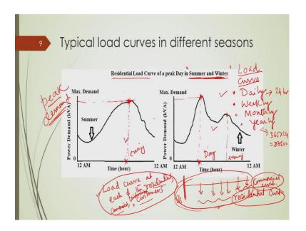
Now, we have some typical load curves ok. So, first thing that I would like to mention that there are different types of load curve; one is called daily load curve. So, if you plot this load demand for 24 hours duration then it is called daily load curve; then, it is also possible to have weekly load curve, then monthly load curve, then yearly load curve. So, here daily load curve duration is 24 hours ok; yearly load curve this duration is 365 multiplied by 24 hours, i.e., something 8760 hours.
