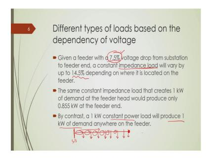
Now one thing one has to understand that as we discuss earlier and we will be discussing in detail in the later part of this course. So, voltage will be varying throughout the year. So, therefore, there might be a voltage drop for a feeder because of this internal impedance of that particular feeder ok. And due to that, it is not possible to have a uniform voltage profile throughout a particular distribution feed it is not possible ok.
