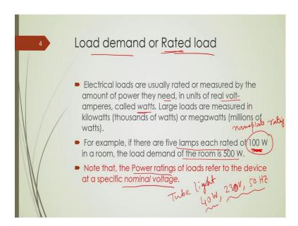
Now, load demand or rated load ok. So, electrical loads are usually rated or measured by the amount of power they need ok; already I mentioned in my last slide and usually it is the real volt ampere or watt ok. So, it is the real power consumption of a electrical appliances ok. Now large load are measured in kilowatt or megawatt, ok.
