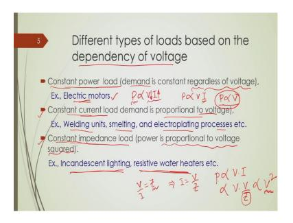
So, based upon this dependency of the voltage, we can categorize the loads in different types. There are certain loads who consume constant power irrespective of the supply voltage ok. So, they consume constant power irrespective of the supply voltage example is electrical motor.
