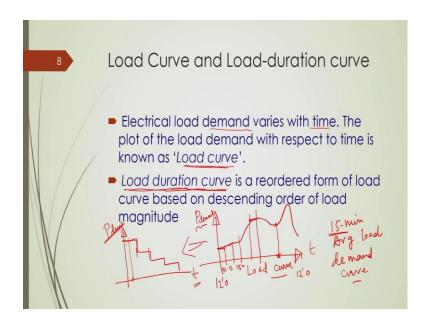
Now, at this point one has to understand that load is a time varying parameter; it continuously varying with time because at what point of time we are using what number of appliances that depend upon our need and that does not remain constant throughout the day and that is true for all the different types of customers.
