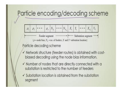
This is a special type of encoding decoding technique, encoding decoding scheme. We have used instead of designing direct information, we have some indirect encoding technique where we have some it is called cost biased encode encoding techniques. So, each of the nodes which are which need to be connected with the new network will have some bias value and this bias value will be updated iteratively.
