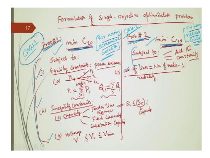
So, this problem 1 is minimization of this cost function under this constraints, we have 1, 2, 3 constraints and also in addition to that we have radiality constraints. So, this is radiality constraints ok, similarly this is what this problem 1 or case 1 ok.
