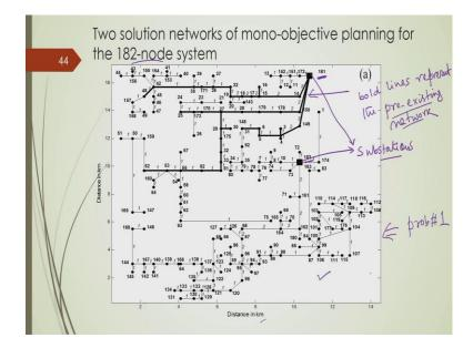
So, this is 182-node system, where you can see these bold lines. So, bold lines represent the pre-existing networks ok. So, here at 182-node at node number 181 and at node number 182 we have substation. So, these two are substations ok and substations locations are specified at node number 181 at node number 182.
