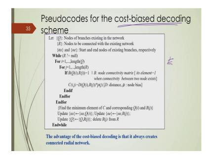
And, from this bias value with the suitable decoding scheme which is mentioned over here which is called cost biased decoding scheme, we get the a total network topology or total network structure of a network and that will make your radiality constraint satisfied ok. It always gives a radial network. So, I will not discuss this in detail, if you have further interest you can go through this algorithm ok.
