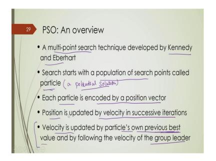
So, PSO is a population based algorithm; that means, it is a multi point search technique. Now, what is that basically? The iterative algorithms can be classified into two types: one is point-to-point search technique, it means that you start with any initial guess and then you update it in the next iteration. But, this PSO or genetic algorithm, these are population based search technique and that is why they are multi-point search techniques.
