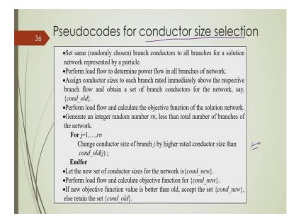
Also, this is how we can select the conductor size, we for each of the branch we assign some set of conductors then we also make some heuristic idea. So, that for each branch or line this line capacity constraint would be would not be violated ok.
