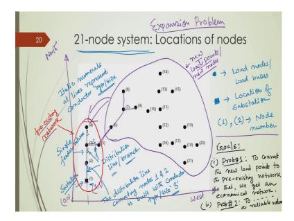
So, let us start with this 21-node system. This 21-node system is having these black dots. So, these dots represent load nodes where we have some load demand or load nodes or load buses ok. So, here we have some load demand and this symbol is representing the location of substation; location of substation. So, here you can see here we have at bus number 1 bus number 1, we have substation located ok and this is a single feeder network.
