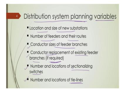
Now, we have some planning variables or we have some decision variables which we need to determine through an approach ok. And what are the planning variables we have? We have to decide about this location and size of the new substation, as well as the capacity addition of the existing substation.
