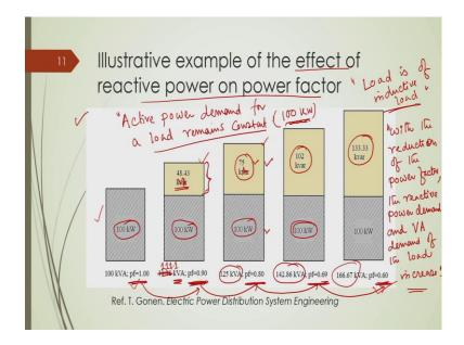
So, and finally, we have shown you, I have shown you an illustrative example for a typical case, in which, suppose, keeping this active power constant or keeping the active power generation constant for a particular generator, who is generating or you can eventually consider that for a substation, from where you are feeding power to the loads or customers.
