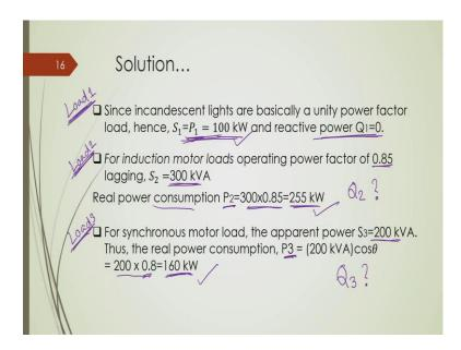
Now, as I have shown you, so this incandescent lamp light which is load 1, this is our load 1; which operates at unity power factor, so it consumes 100 kilowatt and reactive power consumption is 0, ok. Here P 1 is corresponding to the active power demand of load 1 and Q 1 corresponds to the reactive power demand of the load 1. Similarly, here, this is for load 2, which gives you the induction motor loads operating power factor 0.85 and its kVA demand is given as 300.
