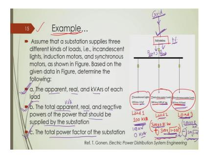
So, before that, I will show an example, numerical example to you. This example if you look at, we have a substation here and in a particular feeder, we have three different types of loads; this is load 1, this is load 2, and this is load 3, ok. And it is mentioned that how much this load 1 is; so load 1 is of a 100 kVA and it operates at unity power factor, power factor is equal to 1.
