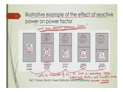
And there is a case also, if we keep this, keep the volt ampere flow from a substation constant and the load power factors are getting deteriorated, then you can see eventually the flow of active power will be get reduced, ok. So, these are nice examples to understand that effect of this power factor on the operation of a typical distribution network and the requirement of reactive power compensation locally, ok. So, these illustrative examples clearly show.
