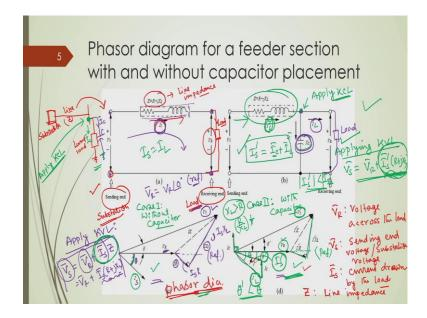
You can see that these three are discussed, one is that reduction of this line current, which is visible over here; another is improvement of this voltage profile, so that you can eventually compare this voltage drop or the difference of voltage of this receiving end voltage and the substation voltage for these two cases. Then you can understand this difference of voltage of the sending end side and this load end would be lower, if we have a capacitor placed in parallel to that plot, ok.
