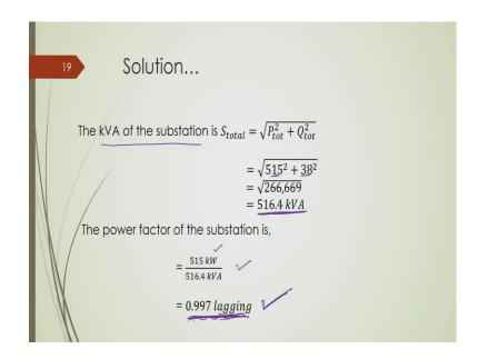
Now, with this, we can find out this total kVA demand which is supplied by the substation, which is coming out to be root of this active power demand and reactive power demand, which is coming out to be this, ok. And we know this active power that needs to be supplied by this substation is 515; we know the kVA demand which needs to be supplied by the substation is 516.4.
