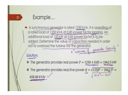
Now, we have another example, this example is of a synchronous generator; this example is of a synchronous generator, which is rated 1250 kVA, which is rated 1250 kVA, ok. And it is operating at a rated load of 1250 kVA at 0.8 power factor lagging ok, at 0.8 power factor lagging. An additional load of 150 kilowatt at 0.8 power factor, this is also lagging; this should have been mentioned, this is also lagging; is to be added to the generator ok, to the generator load.
