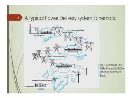
So, this is a typical power delivery system acknowledge this figure from this Lee Willis book you can see that this is the generators then we have this transmission network, these are basically typical representation of transmission line towers and they are having you know transmission lines connected to it transmission conductors connected to it.
