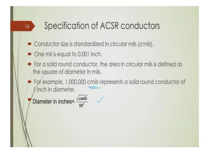
There are some specification by which we differentiate one type of conductor to the other conductors. Normally cmils is one of the definitions. So, this is how we can convert cmils to diameter in inch.
