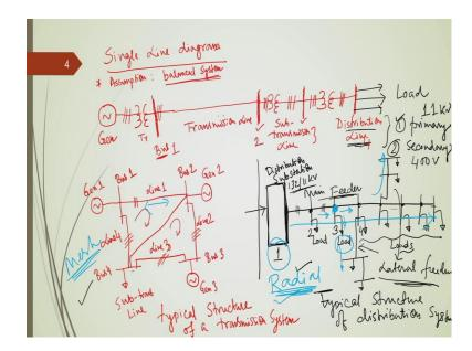
So, first let us discuss single line diagram, what is single line diagram? So, as you know I hope that most of you have some fair idea about this three-phase electrical system. You know that as long as we consider the system is balanced we can represent a three phase system in a single phase equivalent form.
