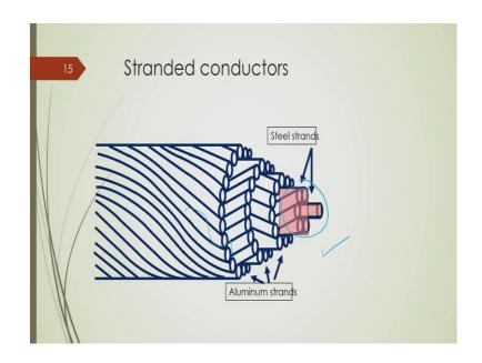
This is the stranded of a conductor; this is how it looks; we have the stranded conductors; this is the steel strands which we use for tensile strength of the conductor and this is how different strands aluminum strands are used to flow this power.
