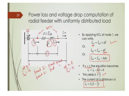
Now, we apply KCL; we apply KCL at these two points; one is point 1 and point 2. So, point 1 is basically you know point 1 is the starting point of this, start point of this infinitely small section and point 2 is the end point; and you know distance between point 1 and point 2 is dx ok.
