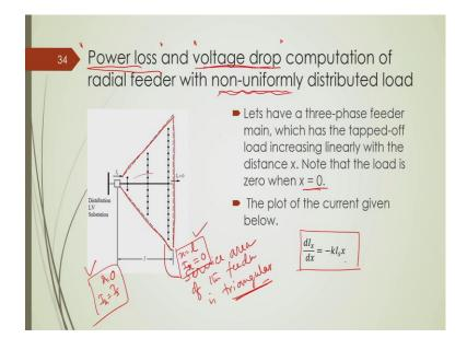
Now, I will also talk about power loss and the voltage drop expressions for a uniformly distributed load. This is not non-uniformly distributed load, but for a uniformly distributed load, but having the service area of triangular ok. So, here the service area, service area of the feeder is triangular and load basically is uniformly distributed.
