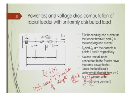
Now, what we can do? So, whatever I discuss and you also know that these are basically you know varying with the length. So, this current is basically I x is function of x ok. So, this current is or I should say that load current is function of sorry function of length ok.
