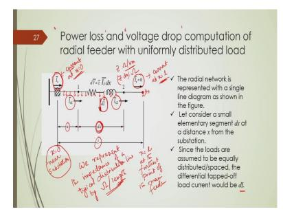
Now, in order to determine this power loss and this voltage drop for typical that feeder, which is having uniformly distributed load and rectangular service area, what we will do? We will consider a typical single line diagram of this feeder; this gives you the single line diagram. This is the total length, this l is the total length and this x is basically providing way you the variable length.
