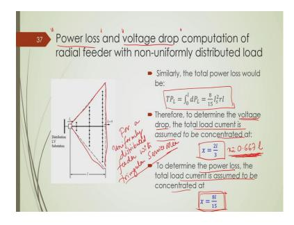
And similarly power loss will come out to be 8 upon 15 I square rl ok and; that means, for a triangular service area of a uniformly distributed feeder, for a uniformly distributed feeder with triangular service area, you can assume that low total load current concentrated at two-third distance of the length.
