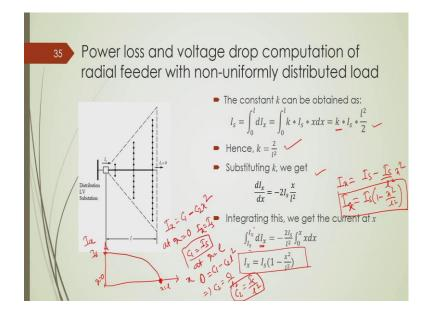
Now, again this we can also determine if you plot this characteristic how this current or the load current will vary from the substation to the furthest point. So, here also we have two boundary conditions that, at x is equal to 0, I x is equal to I s; x is equal to 1 I x is equal to I x is equal to 0. So, these two are boundary conditions, say as similar to the previous example, but here the service area is triangular that is the only difference of that with respect to the previous example ok.
