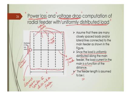
Now, I will go to some analytical approach to determine these two important factors; two important factors of a typical distribution feeder; one is power loss; another is voltage drop ok. These are also the limiting factors, these are also the limiting factors through, which one should decide that how much loading we should allow in a particular feeder or how many numbers of feeders, should we use and should we go for this capacity additions of the substation and all, ok.
