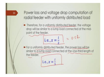
So, this is alternatively represented like this for a uniformly distributed feeder the voltage drop will be similar to the lump load connected at the midpoint of the feeder ok. Now, for a uniformly distributed feeder the power loss will be similar to the lump load connected at the one-third length of the feeder ok. So, that is somewhat new for this type of analysis ok.
