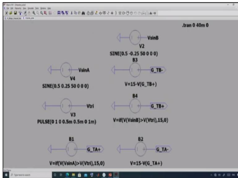
Now, how I have obtained this file that is using this simulation which generates the gate pulses. So, it has got these two references your  $V \sin a$  for leg A and  $V \sin B$  for leg B and this generates your triangular carrier and this is where the comparisons are taking place whether the reference is greater than the carrier or not and accordingly the pulses are generated.
