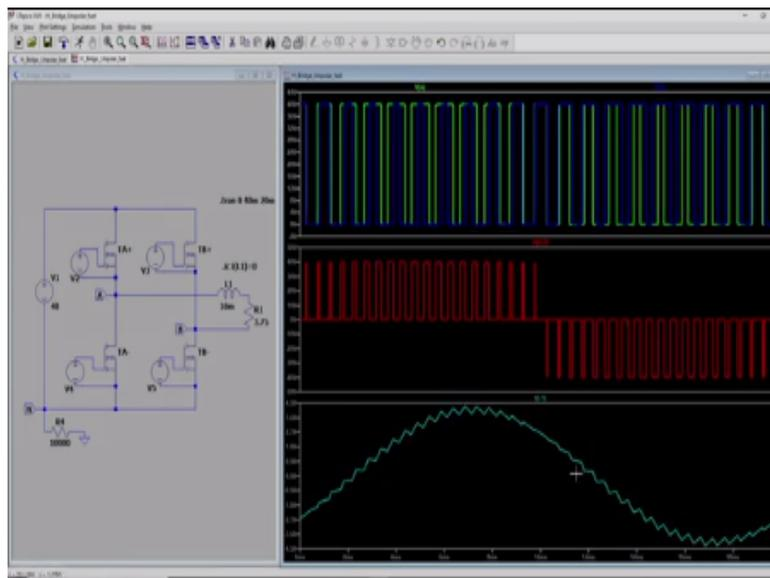
So, when we run this simulation, so, this is what you will obtain. So, what I have shown here is this leg voltage  $V_a$  and then this leg voltage  $V_b$ . So, you can see here that whenever the voltage is positive means the reference voltage is positive your  $V_A$  n pulse width of being
