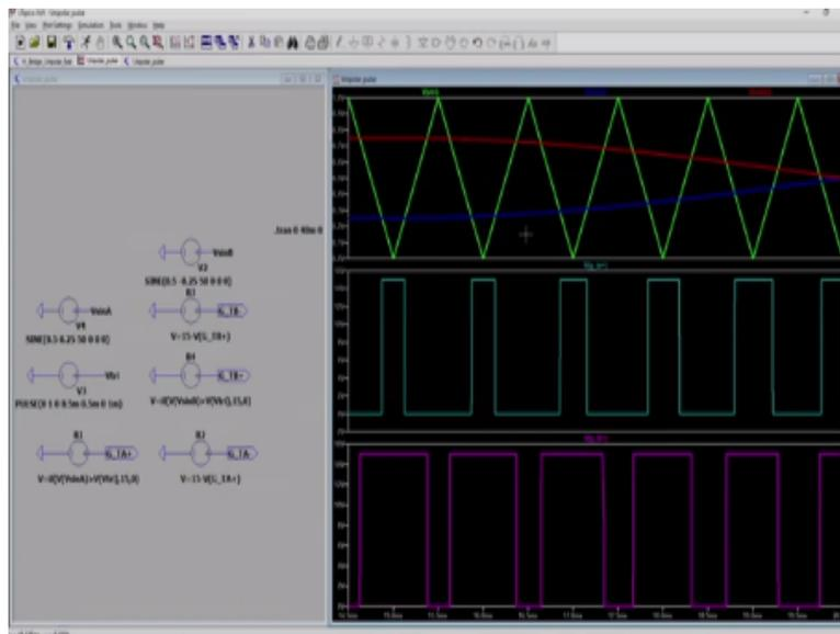
So, now, if I run this, I wanted to show you So, this is the simulation for generating the gate pulse and I have just run the simulation. So, this is your triangular career waveforms this is what is generated and then this is the reference for your leg A; the blue one and this red one is the difference for leg B. And then these two are the gate pulses which are generated for switch TA plus and for the switch TB plus.
