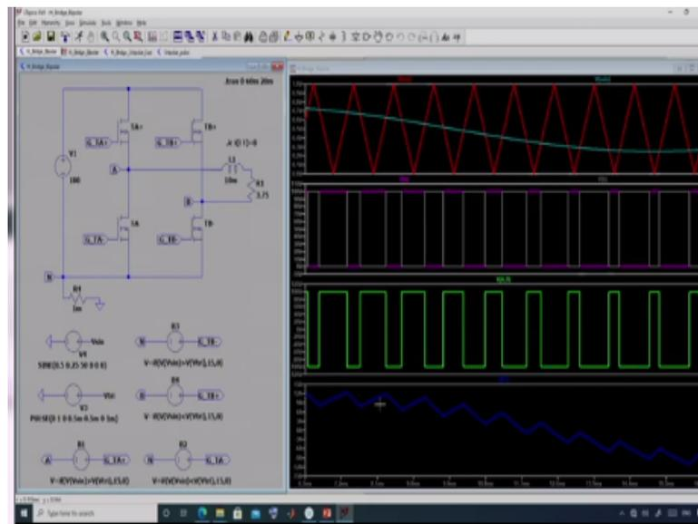
So, now, let us look into the simulation of these H bridge converter. I have simulated both the Unipolar PWM and bipolar PWM to show you whatever we have discussed till now in H bridge you can simulate it and you can see the waveforms and that will also help you in designing the converter.
