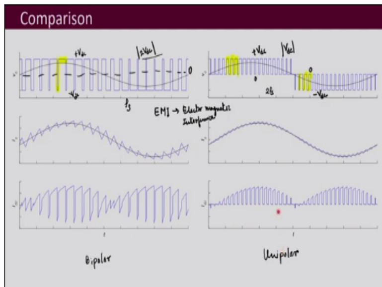
So, these two waveforms we have already seen. So, this is your output voltage waveform for bipolar PWM and this is for these are all the waveforms that we had obtained for Unipolar PWM. So, this is for your bipolar PWM and this is for your Unipolar PWM waveforms. Now, here what you see is that this output voltage over here is varying between minus  $V_{dc}$  to plus  $V_{dc}$ . So, this was your 0 and it varies from minus  $V_{dc}$  to plus  $V_{dc}$ .
