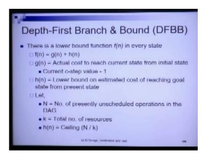
So we said that g(n) is the actual cost to reach the current state from the initial state and h(n) is given by ceiling N/ K what is ceiling N / K N denotes the number of presently unscheduled operators and K is the number of resources so N by K tells me the minimum amount of time that I will require to schedule the rest of the nodes this is how solution will progress.
