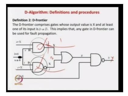
That is if you have just gone for this non modified case ten what is the idea. So, if I gone for non modified case then you have these two gates in the D frontier this gate and this gate in the D frontier. Now it is up to you, whether you see that this gate as the D frontier or this gate has a D frontier to propagate the value of the fault. Now, once you have selected this gate for all propagation then this is related. But there is option one and option two.
