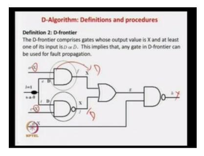
So this X can be controlled in such a way, so that these effect of D and here D' can be propagate the output of this gates which comprises the D frontier.
