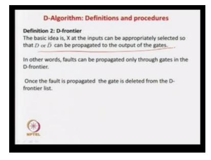
So, that is what actually we say that whenever I gate is in the D frontier then only it can be used for propagating the value of the output of the circuit I am sorry I mean fault effect of the circuit. That is what is the basic idea, the basic idea is that X at the inputs can be appropriately selected, so that D or D' can be compared to the output of the gates that is the basic idea that is.
