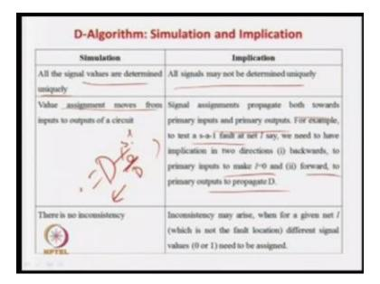
So, simulation primary inputs you give 1011 in the circuit and then you compute the output, so that is very simple. So, in case of implication what we will do it is not a unidirectional flow that will not flow from state this one to input and output. But, there what we will do we first find out the some points we find out some fault, fault is there then sensitize it then we find out the D frontier.
