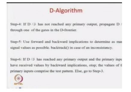
This one so that is that is all the definition we require for knowing the D algorithm and next what we will study actually the D algorithm in detail.
