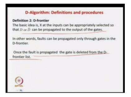
So we can if there is a gate in the D frontier then we have a scope that we can state this value approved lately or accordingly. So, that the fault effect can be propagated through the gates in the D frontier. So, once it is very important, so once the fault is propagate for that this propagated that is say fault is propagated by making this as one then this one will not no longer be in the D frontier.
