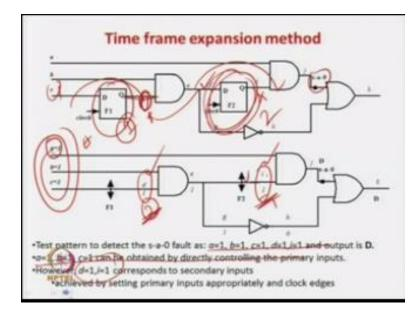
If you look at it so we require to control these two one and also these two one so now they ask that how many clock pulses on patterns you will be required to do this the property says that if the maximum depth is 2 so you can do it in two clock pulses and two inputs.
