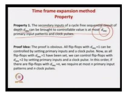
So very obviously it is said that the secondary inputs of cyclic sequential circuits of depth this can we brought in their control in utmost these sequential primary inputs and pattern so therefore if you have a circuit with 10 flip flop of having sequential depth 10 so you require 10 clock pluses and 10 patterns to set the virtual primary inputs and in 11<sup>th</sup> period you require to give the primary inputs and that will solve your problem okay.
