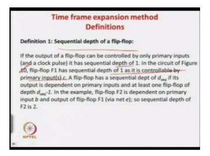
If you look at it so the if the output of a sequential flip-flop is direct this one is 1 then this circuit of figure last figure if you take then either sequential depth of 1 that is directly control by C that is 1.
