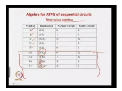
So by adding one extra symbol that is actually 0 < x we got that in case of symbols of ATPG only one pattern or at least one level of competition was less required, so nine valued algebra are equal use this sequential circuit that is 01,1 D and D prime these are all from rows five value algebra, but now we are added some more 0x that is normal case 0 fault case unknown G1 normal case 1 fault case are known F 0 normal case x fault case 0.
