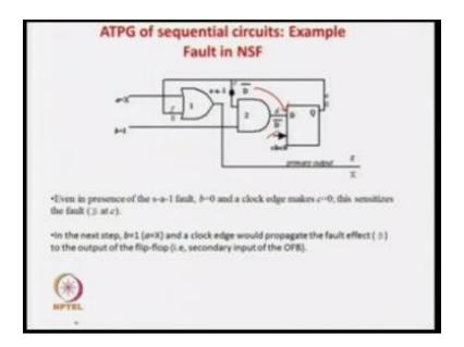
Next you are applying A X = 1, X = 1, B = 0 so your fault effect is propagating to output but the output is you cannot observe so third step what we do again we put a clock edge so that it comes out indirectly but a your primary output.
