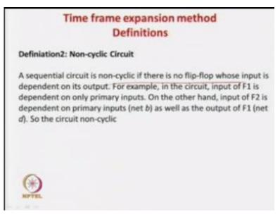
A sequential circuit is non cyclic if there is no flip-flop whose primary input is differ was input is depended in out for example if these.
