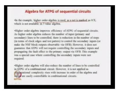
So that is what is the required in the last example higher order algebra this one so which is required to reduce the number of competition or only one test pattern can do it and this is not available in a five valued algebra, so that is why we sometimes we require to go for higher order algebra that is 9 value algebra so higher order algebra improves the efficiency of sequential circuit testing because you require less number of states for the competition.
