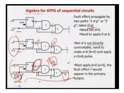
So that is the more difficult if you are considering faults at the next state function block competitive output function block but for all the cases I am like combinational circuit you have to indirectly control virtual and secondary inputs and indirectly observe the secondary output that is what is the basic conceptual difference so in case of sequential circuit more than one test patterns may be required to tested fault.
