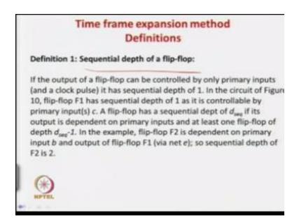
Some other mechanism so that is what is very much require and we will see how to do that but time frame expansion method okay now so just to very simply definition so 1 is call the sequential definition of flip-flop so the output of a flip-flop can be controlled by only primary inputs and clock pulse then the sequential depth of 1 that is.
