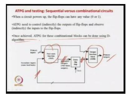
And somehow you should observe them indirectly similarly for the output block you can observe directly for this part no problem but somehow you should control this indirectly so that is what is it says so one state is achieved then ATPG for this combination blocks can be named D algorithm.
