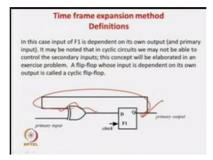
You consider this circuit this is a sequential circuit because his output is depended on its this one this is look at feedback so his output is depended on its owing so that is actually a cyclic definition but if you look at this flip-flop. (Refer Slide Time: 46:22)
