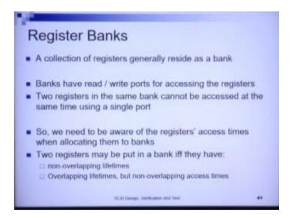
But typically registers in recital a large register file or a bank say in a in a risk machine and these register bands so the register inside these register bands can be accessed through read/write ports so a collection of registers generally reside inside of guy banks have read write ports for accessing the registers to registers in the same bank cannot be accessed at the same time using a single port so if you have two registers in the same register bank you
