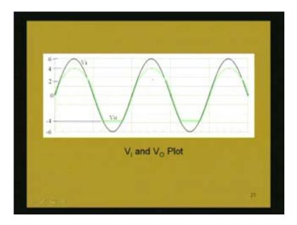
From 0 to 2 input and output is same and at input 6 volt, output voltage is 4 volt we have found out and again when it is less than 2 it will not conduct. It will not conduct till the negative half cycle when the magnitude of the input voltage is greater than 4 volt. That means if it is more negative than -4 then only it will conduct and the voltage will be -4 volt. It will be constant voltage drop. When  $V_i$  is again less it will not conduct. Input and
