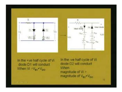
Similarly other diode conduction is in this direction from bottom to top. So the diode drop  $V_{DO}$  will be also having the same polarity that is positive here, negative here. This is  $V_{DO}$  and the other voltages battery  $V_{B1}$  and  $V_{B2}$  are as it is we have drawn and these are ideal diodes. We have to find out what is the output voltage for a given sinusoidal voltage  $V_i(t)$ .
