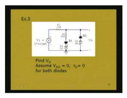
In the positive half cycle if you consider a portion when  $V_i$  is less than 2 volt, for zero to 2 volts, we find that D1 and D2 both are OFF; both are not conducting. Both are reverse biased and both are not conducting. What will be the output voltage? Output voltage is equal to the input voltage exactly equal since these are ideal diodes in consideration.
