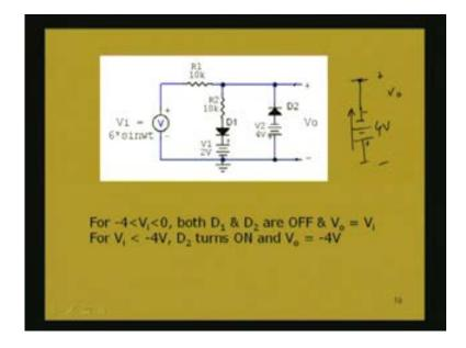
So  $V_o$  is -4 volt when the diode D2 is turned ON. Combining all this we can now draw the output voltage waveform versus input voltage waveform. Input is this one, black one. Output will be the green one.
