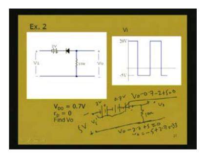
So -2.3 volt you will be getting at the negative side. We get zero voltage in the positive half cycle. It will not be conducting. Resistance R or 10 K will not have any current rates. This voltage is zero in the positive half cycle. But in the negative half cycle the voltage will be clipped at -2.3 volt. This kind of an output voltage waveform we will be getting for this circuit.
