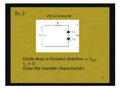
$V_{DO}$  is the diode drop in the forward direction. Because in the forward direction Zener diodes can conduct and like normal diode it will be having the voltage drop  $V_{DO}$ . If you give a sinusoidal voltage what will be the output? Whenever the input voltage is in the positive half cycle this Zener diode will be reverse biased. Positive will be reverse
