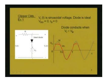
Here you notice that we are still assuming that the diode is ideal without any voltage drop when it conducts and resistance being zero but now we consider the diode having the voltage drop  $V_{DO}$ . That means we consider another example where we have a diode which has an equivalent constant voltage drop model. Let us see an example of a clipper circuit using a constant voltage drop model of the diode that means a diode which has  $V_{DO}$  equal to say around 0.7 volt for silicon.
