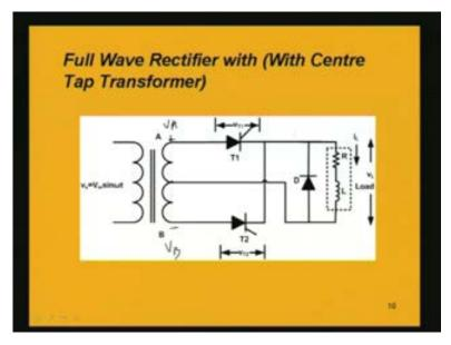
If we consider the voltage  $V_A$  here and  $V_B$  here,  $V_A$  and  $V_B$  will be just out of phase by 180 degree and so  $V_A$  will be like this and  $V_B$  will be like this. They are out of phase by 180 degree. Now what will be the output voltage? That will depend upon the current
