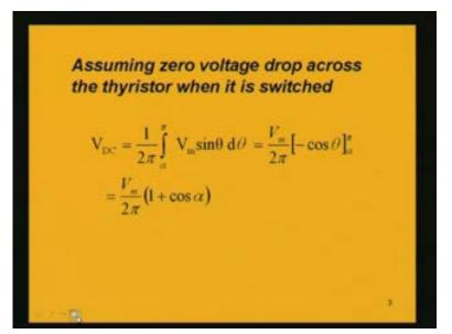
We can find out the voltage values. Assuming zero voltage drop across the thyristor when it is switched or fired we can find out the DC value of the voltage, DC value or average value because we are having a rectifier. It is a half wave rectifier.
