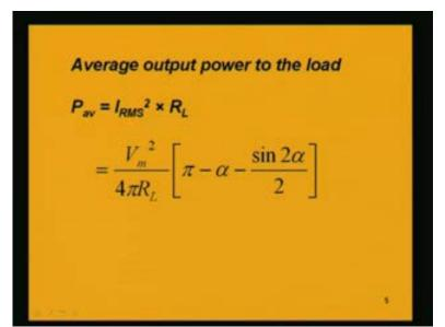
If we want to find out the average output power to the load, output power is nothing is  $I_{RMS}$  square into  $R_L$ ; average output power to the load that is obtained as  $I_{RMS}$  square we have found out. Replacing this expression here and multiplying by  $R_L$  will cause the square in the denominator of  $R_L$  to vanish. What will be here is  $V_m$  square by 4 pi  $R_L$  into pi minus alpha minus sin twice alpha by 2.
