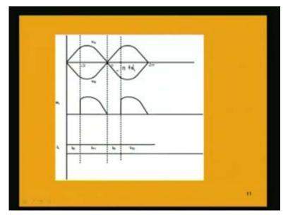
We are getting the voltage across this load following the voltage at the input that means at the secondary side.
