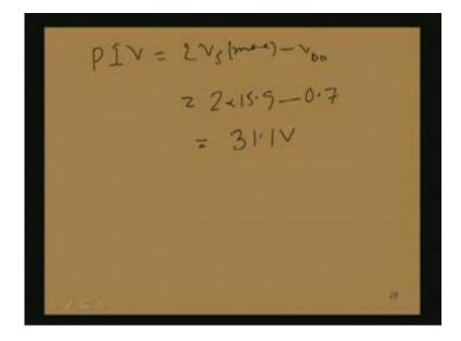
In this way we can solve this problem and whatever you do, you must assume either the constant voltage drop model or ideal diode. In this example it is given that it is constraint voltage drop; so we can proceed like that.
