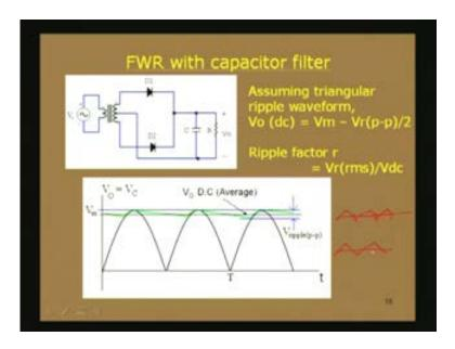
That is why  $V_m$  minus  $V_r$  peak to peak by 2 gives you that DC voltage for this full wave rectifier with capacitor filter. If we consider the whole conduction and non-conduction of the diode, the diode is conducting only for a very small portion. That is for a very small time  $T_1$  and it is non-conducting and it is only because of the discharging of this capacitor that we are getting the output voltage. It is for capital  $T_2$ .
