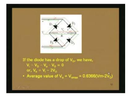
It is  $2V_D$  because in the positive half cycle the current will be flowing through  $D_2$ , then R and then  $D_4$ . There is drop here. There is drop here also. So two voltage drops will be coming into the picture. The diode drop  $V_D$  will have to be multiplied by 2. That means
