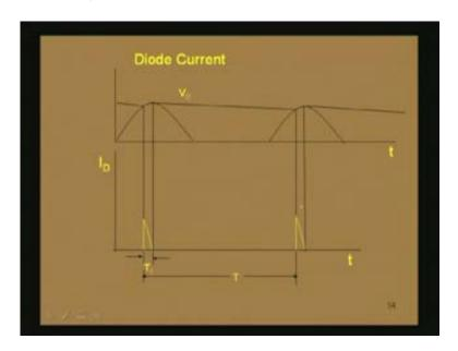
This diode conducts for a very, very small time. That is why it is called the surge current. For example if we consider the whole time period, only for a small portion  $T_1$  it is conducting. If we consider our power supply which has 50 Hertz frequency supply, the time period will be 1by F, 1 by 50 Hertz which gives you 20 millisecond.
