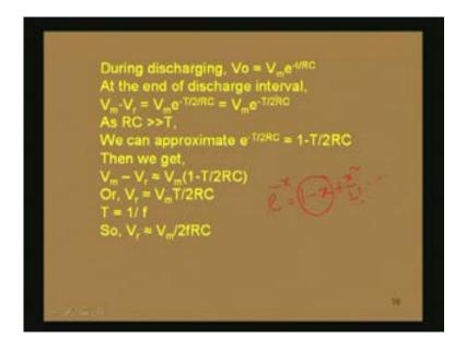
Then we get  $V_r$  equal to  $V_m$  T by 2 RC;  $V_m$ ,  $V_m$  cancels. This term will be remaining and we know the time T is equal to 1 by frequency. We can write  $V_r$  that is the ripple voltage is equal to  $V_m$  by 2 f RC replacing T by 1 by f.
