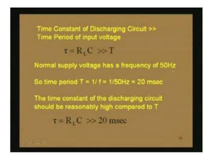
The time constant of the discharging circuit in the rectifier should be reasonably high compared to T means we should chose value of tau very, very great as compared to 20 millisecond. It should be sufficiently high so that we get overall almost constant DC voltage. It should not fall of drastically. Similarly if we consider full wave rectifier with capacitor filter there will be capacitance which will be connected in parallel with the load resistance.
