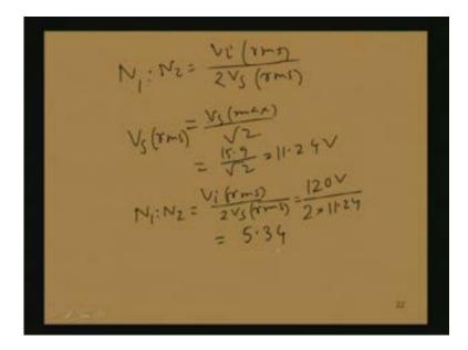
PIV of the diode can be found out. If we look into the circuit what will be PIV?  $2V_S$  peak value minus this drop  $V_{D0}$  will be the peak inverse voltage of the non-conducting diode. So PIV is  $2V_S$  max minus  $V_{D0}$ . So 2 into 15.9;  $V_S$  max is 15.9 minus 0.7 whole drop is given to you; 31.1 volt. This is the PIV and the turns ratio we have found.
