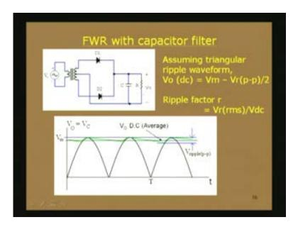
Here better approximation to DC will be obtained because if you consider the input voltage which is rectifier in full wave rectifier in the both half cycles again we are getting
