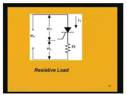
We will understand how the phase control is being achieved using resistive load and then we will also discuss about an inductive load. Now in this circuit we are applying the AC sinusoidal voltage which is  $e_s$  and this thyristor is connected to the resistance R and let us take the voltage across this thyristor as  $e_T$  and R is the load and the voltage across this load R is say  $e_L$ .
