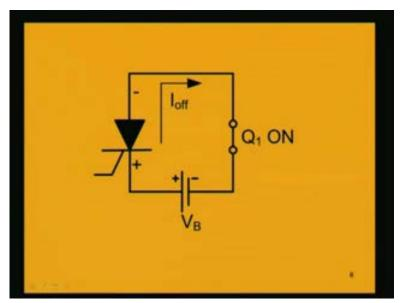
Due to this current flow when the transistor is ON, the polarities of the thyristor are becoming positive to cathode and negative to anode. As we see here the transistor is ON. It is like a very short circuited part. So, conduction is taking place in the transistor. That is why current is flowing and making this thyristor OFF by making the polarities of the anode and cathode like this; just opposite or reverse biased. This is the forced commutation which also makes the thyristor turn OFF.
