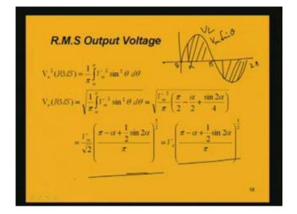
But the consideration of the whole period is to be done because the root mean square value when we find out, we are finding out the root mean square value of the output voltage  $V_L$  for this whole cycle between zero and 2 pi and out of this whole cycle from zero to 2 pi we are finding out from alpha to pi because from zero to alpha there is no conduction. The voltage will be zero. Only the voltage will be here and again here.
