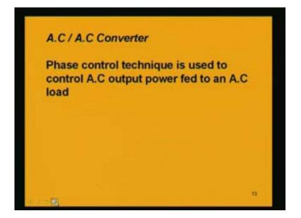
The AC to AC converter is a device where the phase control technique is used to control the AC output power fed to an AC load. We are considering a load which is getting an AC power. The AC to AC converter using thyristor does the controlling of the AC output power to an AC load. How it does so?
