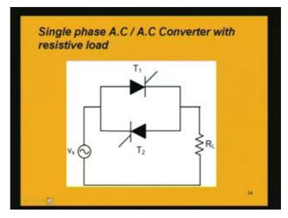
To understand that let us consider a circuit having two thyristors  $T_1$  and  $T_2$  back to back like this, as is shown in figure. We are considering single phase AC to AC converter. We
