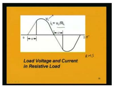
RMS value of the output voltage when I find out output voltage is there or available for whole period from zero to 2 pi. There are in between non-conducting periods from zero to alpha but we are finding out the RMS value or root mean square value. For the whole period we will have to divide it by 1 by pi here because we are integrating between alpha to pi for one half cycle.
