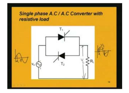
In the whole input waveform cycle, for half of the period thyristor  $T_1$  is conducting and for the other half thyristor  $T_2$  conducts not for the exact half but less than one half. It is firing at an angle of alpha; so, basically the thyristor is ON from alpha to pi. The thyristor  $T_1$  if we consider it is firing at an angle of alpha and it continues to conduct till pi.
