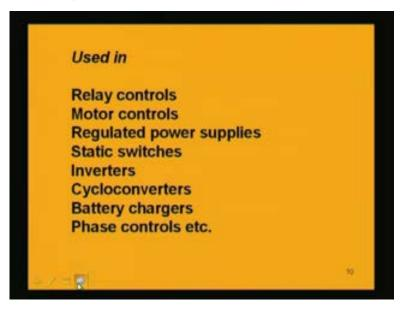
Some typical examples where we use this SCR or thyristor are relay controls, motor controls, regulated power supplies, static switches, inverters, cycloconverters, battery chargers, phase controls, etc. Typically we will find in control applications, motor control using thyristor, we can control various other devices. We will find that these thyristors are used in power control or motor control or relay control, etc.
