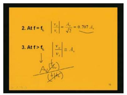
Ultimately we will get  $A_v$  into f by  $f_L$  in the numerator. This term is there in the denominator also we will get f by  $f_L$  and these two cancel. So we get a constant voltage  $A_v$  that is 1 plus  $R_f$  by  $R_1$ . In the high frequency region when the frequency is greater than the cutoff frequency we get a constant voltage gain and the signal is totally allowed. It is passed with a gain.
