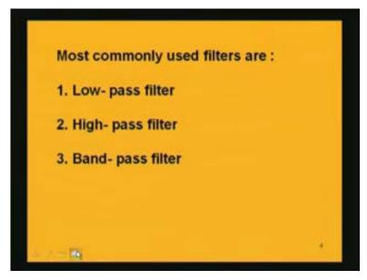
For example, if we take a low-pass filter, in an ideal low-pass filter, the input signal frequencies at the lower range of the band are allowed to pass and it completely stops after a desired cutoff frequency say  $f_{\rm H}$ .
