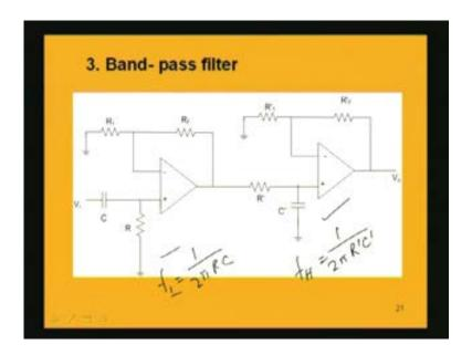
This will determine the high cutoff frequency  $f_H$  and that will be given by 1 by 2 pi R dash C dash and this is giving you the high-pass filter.
