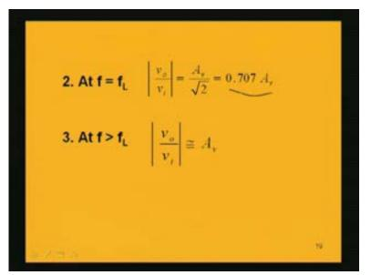
We get at f is equal to  $f_L$ , the value of the gain magnitude is  $A_v$ by root 2 and that is 0.707 times  $A_v$ . This is again known as 3 dB frequency, because 20 log 0.707 will give you 3 dB. The gain is increased to 3 dB of the value of  $A_v$ .
