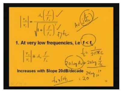
This is a constant term so the slope can be obtained from this part. If frequency is increased 10 times, it will be 20 log 10 to the base 10; it will be 20 for earlier frequency  $f_1$  and then we are taking say 10  $f_1$ . In between these two frequencies, if we take this part it will have a 20 dB per decade slope. In the low frequency region when the frequency is increasing we are having an increase of gain and a positive slope is signifying that and that slope is 20 dB per decade.
