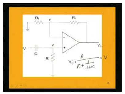
Here we have to find out what is the voltage at this point which is the non-inverting terminal and by the same analysis we will find what is V, voltage division is taking place. Input voltage is  $v_i$ ;  $v_i$  into R divided by R plus 1 by j omega C and that is equal to v. Here this voltage is our interest actually. What is the voltage at this non-inverting terminal?
