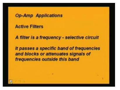
The filter is a circuit which passes a specific band of frequencies and it blocks or attenuates signals of frequencies outside this band. So selectively it passes a particular band of frequencies. Depending upon which band of frequencies it allows and blocks the other band of frequencies we have different types of filters, like we have low-pass filter, we have high-pass filter and also band-pass filters.
