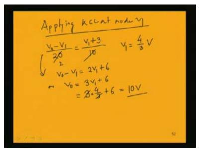
KCL, Kirchhoff's current law we are applying at node, which has a voltage  $V_1$ . So that gives us the incoming current i is equal to the outgoing current, same current but we will find out this expression from the node voltages  $V_0$  minus  $V_1$  by 20 k. Omitting this k because both sides will have the same unit equal to as I have said  $V_1$  minus -3 that is  $V_1$ plus 3 by 10 and we already have known what is the value of  $V_1$ .  $V_1$  is equal to 4 by 3
