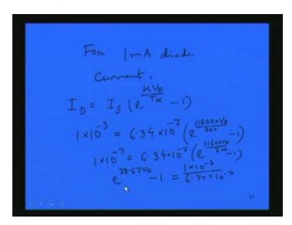
e to the power  $38.67~V_D$  will be equal to 1 plus 0.1577 into 10 to the power 4. We can now find out right side which is equal to 1578. That is e to the power  $38.67~V_D$  equal to this. We can find out  $38.67~V_D$  equal to natural logarithm of 1578 and that is equal to 7.3639. We can find out what is  $V_D$ ? Applied voltage or bias voltage is divide this by this it will be equal to 0.19 volt. For this 1 milliampere diode current, we have to apply 0.19 volt.
