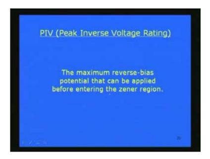
The maximum reverse bias potential that can be applied to the diode before entering the Zener region. PIV of a diode, that rating you have to always remember before applying it under the reverse bias condition. We will be considering a diode but before going to the practical diode let us consider a theoretical ideal diode.
