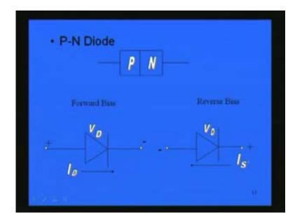
What will be the relationship between the current and voltage in a semiconductor diode? That is an important relationship we must remember. This is given by  $I_D$  equal to  $I_S$  into exponential K times  $V_D$  divided by  $T_k$  minus 1.
