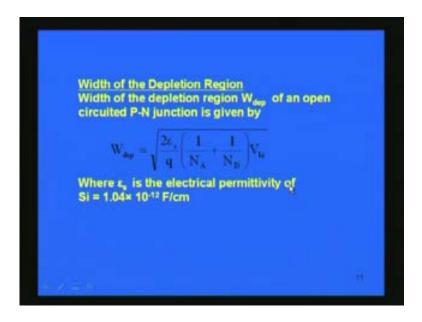
If I consider this silicon material it is 1.04 into 10 to the power of -12 Farad per centimeter. If we know these two expressions we can find out what will be the value of this barrier potential or built-in potential and depletion layer width for a p-n junction.
