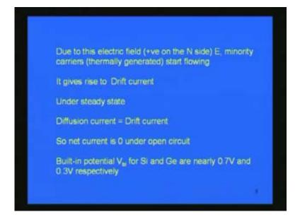
This built-in potential for silicon and germanium are nearly 0.7 volt and 0.3 volt. The barrier potential is such that if we consider from the P side it will be rising and we get a maximum value of this built-in potential which is  $V_{\rm bi}$ .
