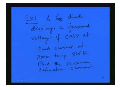
Here you have to assume that diode ideality factor eta is 1. This is given to you. Also you have to calculate the bias voltage needed for diode current of 1 milliampere. What will be the bias voltage to be applied when the diode current is 1 milliampere and also 100 milliampere? These three cases; it is given at 10 milliampere. Then you have to find out for 1 milliampere and 100 milliampere at the same temperature. Temperature does not change. This is the second part of the problem.
