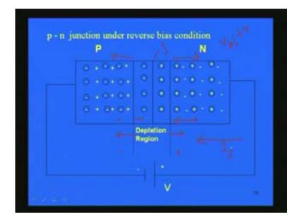
It will be increased if we raise the temperature because you know that increase of temperature will result in production of more and more minority carriers. More and more electrons will be breaking away from the covalent bonds of silicon or germanium and more and more electron hole pairs are created when you increase the temperature. Other than that the applied voltage does not have much effect on this reverse saturation current.
