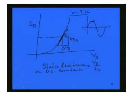
The dynamic resistance or AC resistance is given by del VD by del ID around this Q point that is incremental change in voltage by incremental change in current.
