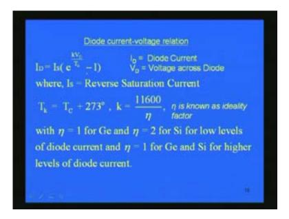
This expression gives the current flowing in a diode when the voltage across the diode or the biased voltage is  $V_D$ . K is a constant given by 11600 by eta. Eta is known as ideality factor of diode. The value of eta is 1 for germanium and 2 for silicon when the diode current is low that is in the lower region of the diode current. These are different values but in higher level of diode current you will be having the same eta value 1 for both
