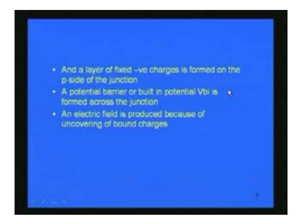
This uncovering of bound charges produced an electric field. This electric field will now act upon the minority carriers so drift current will be produced and under steady state diffusion current is equal to drift current. So net current will be zero under open circuit.
