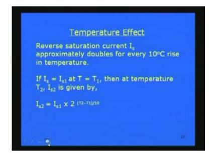
It will be increasing. How much it increases that is actually given by a law that for every 10 degree centigrade rise in temperature the reverse saturation current approximately doubles. That means if suppose at temperature  $T_1$  we have a current  $I_{s1}$ , reverse saturation
