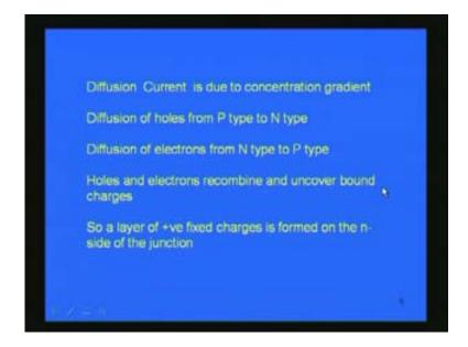
A layer of positive fixed charges is formed on the N side of the region giving rise to a potential and that potential is known as built in potential or sometimes it is named as barrier potential.
