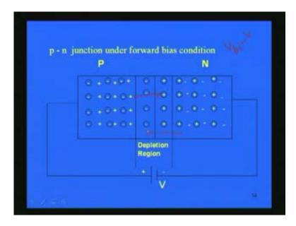
That means when we forward bias a p-n junction there is easier flow of holes and electrons from P and N side. That is the diffusion current will be increasing and with a
