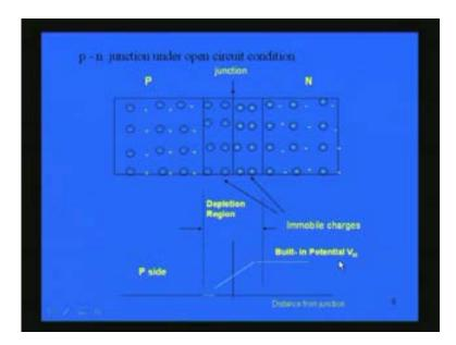
This built-in potential has an expression given by kT by e and natural logarithm of the product of  $N_A N_D$ , which carry their usual meaning, that is the concentration of the acceptor atoms and the concentration of the donor atoms divided by  $n_i$  square which is intrinsic carrier concentration.
