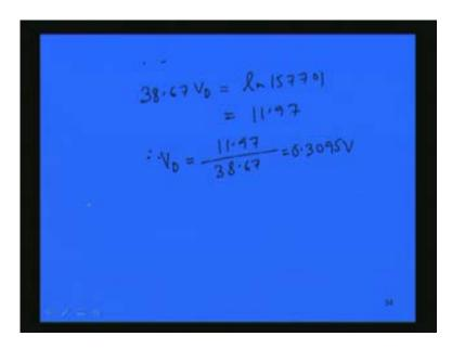
Even if we increase the voltage by less than twice, we are getting 100 times of diode current. For a small change of applied voltage we are getting such a huge current change or rise and that is very, very clear from that characteristic curve also.
