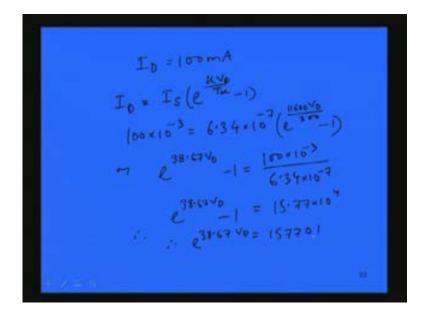
From here  $38.67~V_D$  you take out by taking natural logarithm of 157701. That is equal to 11.97.  $V_D$ , the bias voltage which has to be applied to get 100 milliampere current becomes 11.97 divided by 38.67 which come out to be 0.3095 volt. This much of voltage is required. Notice that we are getting 0.3095 in this. For this 0.3095 voltage, 100 milliampere but for 1 milliampere we had to apply a voltage of 0.19 volt.
