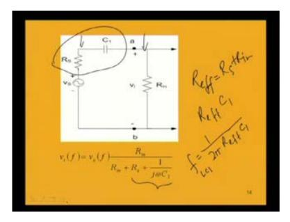
Let us try one problem for finding out the lower cut off frequency due to the capacitance  $C_S$  alone as shown in this figure. In this example we will find out the lower cut off frequency due to the capacitor  $C_S$  alone.
