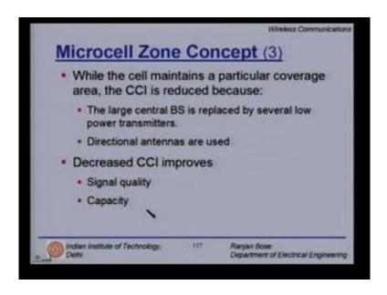
so if we continue the concept of microcell zones while the cell maintains a particular coverage area, the CCI is reduced because the large central base station is replaced by several low power transmitters. we have reduced the power. directional antennas are used. CCI 's are also reduced.
