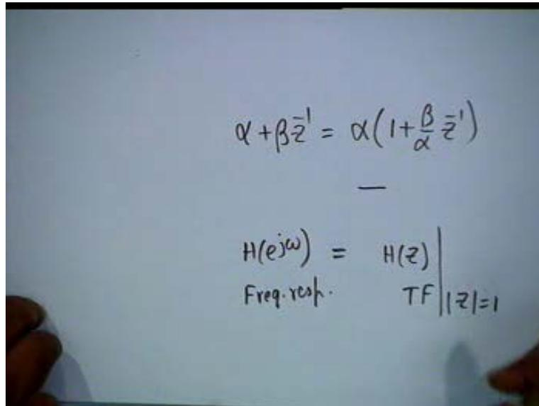
The image shows a whiteboard with handwritten mathematical equations. The top equation is  $\alpha + \beta \bar{z}^{-1} = \alpha \left( 1 + \frac{\beta}{\alpha} \bar{z}^{-1} \right)$ . Below it is a horizontal line. The bottom equation is  $H(e^{j\omega}) = H(z) \Big|_{TF} \Big|_{|z|=1}$ , with "Freq. resp." written to the left of the equals sign.
