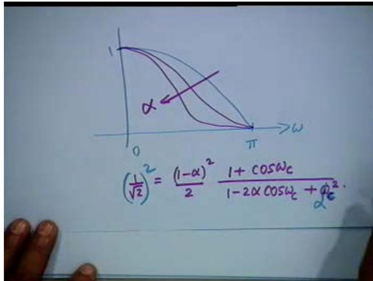
The only parameter for this LPF is alpha. Unlike the simplest FIR which is  $(1/2)(1 + z^{-1})$ , the cut-off frequency can now be controlled by alpha. And if you plot the characteristics, it would be like that shown in the figure. As alpha increases, the characteristic becomes better and better. How do you find the 3 dB cut-off frequency? The maximum is 1.
