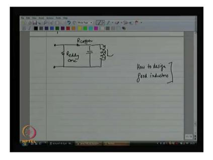
Now, then we went further and we develop the some kind of module for the inductor; we saw the resistance, the series resistance is a series R eddy, the R copper is series resistance; the eddy current create a parallel resistance be with so that is model over there.
