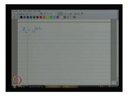
So, these kinds of leads you believe that the wire almost works like an inductor; the inductor impedance increases as frequency increases right; somewhere it rings the bell and we are talking about wire whose resistance increases as frequency increases. So, you know wire is kind of behaving like an inductor.
