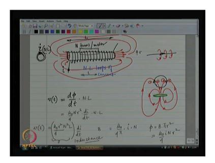
Iron core, let us say and there is winding, copper winding around this core that is your typical discrete inductor. You can also make this core in the shape of a torrid etcetera. So, let us think about this, this is a solenoid. Let us assume that the solenoid is infinitely
