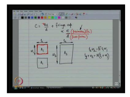
So, the net capacitors now is proportional to the area and there is some additional capacitance, because of the fringing. Now, this fringing capacitance is going to be proportional to what, is it going to be proportional to the dialectic constant yes, is it going to be inversely proportional to the distance between the two plates, yes. What else is it going to be proportional, is it going to be proportional to the area no, take a look or let me draw the top view.
