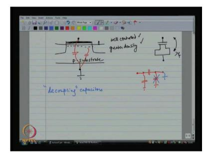
The other well known capacitor is the gate oxide of a Mosfets, so can I use the gate oxide of a Mosfets to create a capacitor, this is actually something which is very very popular. And the reason behind it is that gate oxide, the thickness of the gate oxide of a Mosfets is well controlled and very small, so you get extremely high capacitance density, and you get a much better controlled value of the capstone.
