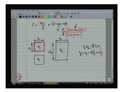
So, the net capacitance, now is proportional to the area, and there is some additional capacitance, because of the fringing. Now, this fringing capacitance is going to be proportional to what, is it going to by proportional dialectic constant, yes is it going to be inversely proportional to the distance between the two plates yes. What else is going to be proportional, is it going to be the proportional to the area no, take a look or let me draw the top view.
