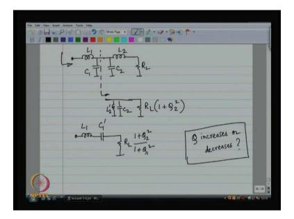
So, let us look at this T match briefly, so it is the same strategy as before, I split up this capacitor C into C 1 and C 2 they are in parallel, and now I have got L 2 and series with R L to an inductor in parallel with the resister, now I am going up. And I make sure that C 2 resonates out with L 2 prime at the frequency omega 0, so I can delete C 2 and L 2 prime both, and now from this point this is what I see.
