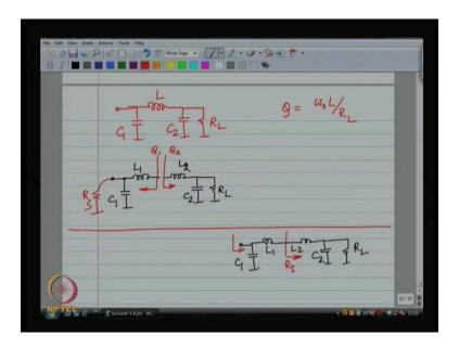
So, this basically tells me that the net cube of my circuit, this was my circuit that we started from, this basically tells me that the net cube is omega naught L by R L, it is almost as if I have a series combination of L and R C 1 C 2 etcetera are accessories. So, that is the net Q of my circuit, is there another way to see this happening, well another way to see this happening is to examine this from the centre.
