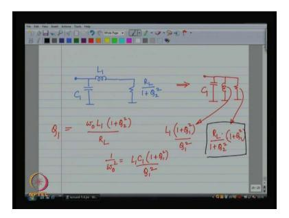
This is what I see at the frequency omega naught, now we can further transform is L 1 is in series with a resistor, so this can be transformed into a parallel combination of an inductor and the resistor. And what is going to happen, this is going to transform into
