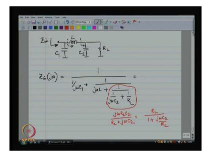
So, my input impedance Z in, that is equal to the capacitor parallel in with some other stuffs, so that is what I am writing down over here, what is the other stuffs it is an inductor in series with some other stuffs. And that is basically a resister in parallel with a capacitor, so the net quantity can be simplified to what, so first of all let us try to simplify this lower most quantity, this is yes, and actually it is never written in this fashion.
