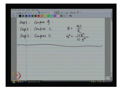
Number 1, compute the Q dot, Q is going to be this, step 2 compute L, what is the relationship between Q and L inductor is parallel with the register, the Q is omega naught L by R L right. So, L is going to be Q times R L divided by omega naught that act a chosen frequency omega naught, and step 3 is compute C we want back words in our derivation in our explanation. So, C is this C is going to follow this equation you know L Q and omega naught, so you figure out what C is all right.
