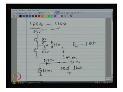
And one of the bands of GSM is from 1.6 gigahertz to let say 1.8 gigahertz numbers might not be exactly accurate, but let say this is the case. So, the cell phone needs to transmit in any channel over the entire band, so the basic station you tell the cell phone at exactly what frequency to transmit, and that frequency could be anywhere between 1.6 and 1.8 gigahertz suppose this quite avoid band.
