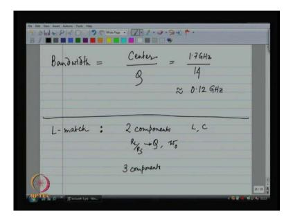
So, what is the band width is the centre frequency divided by Q, so we have got 1.7 gigahertz are center frequency divided by Q is about 14. So, my band width is a little about 0.1 gigahertz that is the total width of the band in which I will be able to transmit reasonably good amount of power, the match is going to be reasonably nice right. The desire band width is 0.2 gigahertz, the band width that I am getting is 0.12 gigahertz which is significantly lesser, so this is my problem right.
