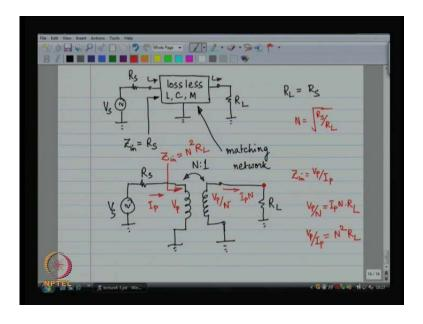
Now, let us consider the following let us say I have a source which has which is in separable from source resistance, and I have a load. Now, for maximum power transfer given R S, R L has to be equal to R S, this is for maximum power transfer, what if R L is not equal to R S, what do you do you given up. Alternatively what we could do is we
