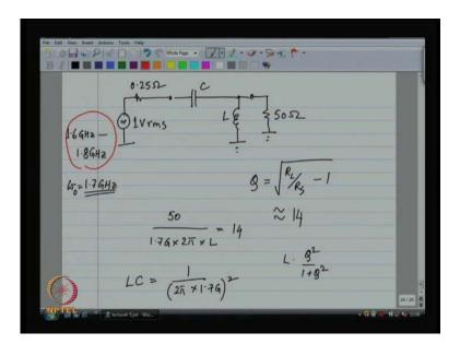
So, this is what I have got, I have got a system which puts 1 volts r m s signal it has a source resistance of 0.25 ohms right. Unfortunately the load is not 0.25 ohms, the load is
