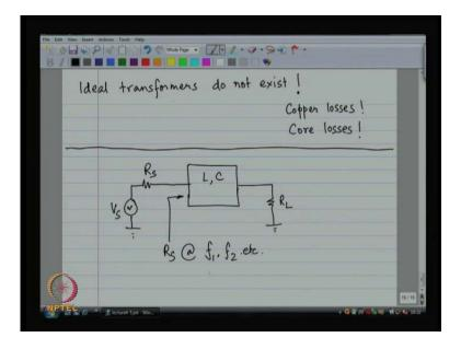
The catch is that I assumed that I have got an ideal transformer, does not exist impossible to make an ideal transformer we going to study transformer later on. But, it is not possible right, second thing is transformers also consumed power, it is impractical to say I am, going to make transformer dose not going to consume power, they are going to be
