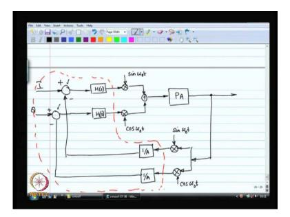
So, this is modification of the previous architecture accommodated for in band and quadrature phase. This is actually a very popular architecture as far as the transmitter is concerned. So, the signals I and Q are directly coming from D to A converter. And, they are a little bit not exactly at DC because it is hard to make the mixer the feedback mixer
