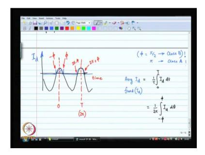
So, this is basically the idea that the power delivered is V D D times I max by 4 though power, but you have consumed is average current times V D D. So, therefore, the efficiency is how much pi by 4 pi by 4 is something like if say pi is 3 then it is 0.75 pi is a little more than 3.14. So, it is something like 77 percent.
