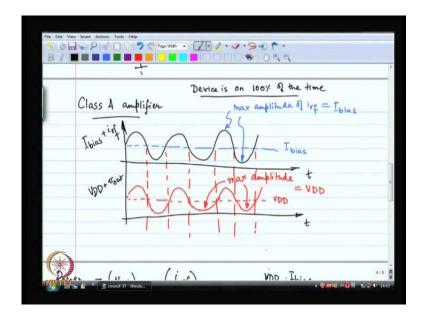
So, let us first discuss class A amplifiers now, class A amplifier is the most straight forward generic amplifier. The class A amplifier is the most straight forward generic amplifier where basically the transistor and the MOSFET that have used over here is in saturation all the time.
