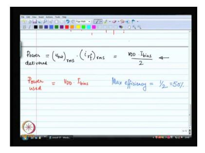
That you can deliver to the load the power deliver to the load is the amplitude of V out actually no it is the r m s of V out times the r m s of I rf. Now, the r m s of V out is equal to the amplitude of V out is V dd.
