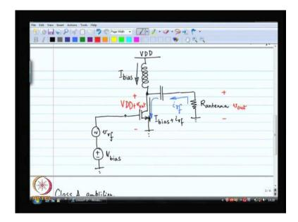
So, the very generic structure which is important for lot of the classes of the power amplifiers is basically something that is looks like this. So, R antenna is the radiation resistance of the antenna.
