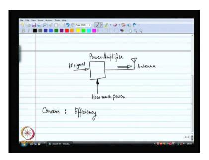
Then you will have some RF signal then you will apply the RF signal to the power amplifier and the requirement of the power amplifier is basically to pump out as much energy as possible through the antenna and broadcast the message.
