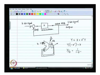
The output is the 1 bit signal and the claim is that the average of the output. So, suppose the H is the filter which has very high gain at d c infinity high gain at b c and low gain at other frequencies does not matter what the gain is at other frequencies, what at d c it is a
