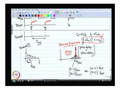
Now, because up and down have the small clutches and because it is impossible to perfectly match to current sources, also note one current source is a source the other is the sink. So, they are not even of the same quality, so one will be made with N
