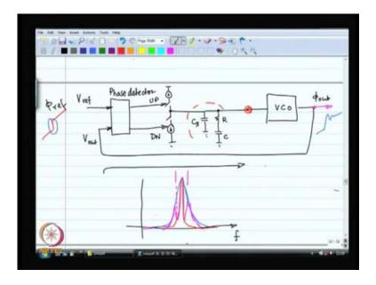
What going to happen if I increased the capacitors, if I increase the capacitance the r c product is going to increase, which means that the loop band width is going to decrease; fairly, simple if I decrease the loop band width, if I decrease the band width of this particular filter.
