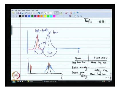
So, let us say n equal to 2, so this is sorry this is the crystal accelerator spectrum and twice this frequency is my v c o spectrum kind of exaggerating, the view put a lot of bad noise are there. Now, the comparison is between the divided output you divide the output
