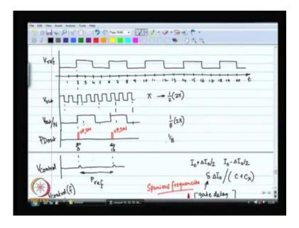
So, next we did a small exercise and we saw, that even when up and down even at perfect lock between, the reference and the divided output even these two are perfectly locked up and down have small pulses of equal duration. And this happens, because of the delay of AND the get as well as the clear operation within the flip flop.
