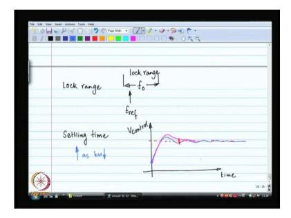
So, phase lock loop has a lot of these properties lock range is one of them. So, the voltage controlled oscillator has a certain center frequency free running that is that is the frequency that it is going to oscillate at and if the reference frequency is anything within the lock range of that. So, if the reference frequency is out, then the voltage controlled oscillator will be able to lock to that reference frequency.
