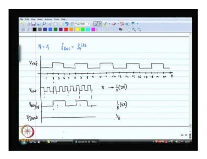
Let us say N is 4 and let us say we are working with the 1 hertz clock f ref is 1 hertz. Just for convenience I want to see what phase detector output looks like, etc. So, as a function of time let me first plot the reference equation the reference voltage. So, the reference voltage probably looks like this.
