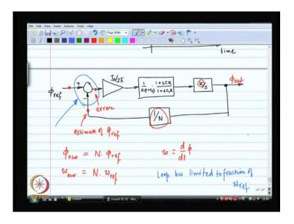
Now, let us move on right is it conceivable this is my phase detector. So, this is the normal phase lock loop what is going to happen if I put a division by N in the feedback path will this loop also work off course this loop will work I mean it has the same dynamics as before it is just that effectively instead of having K by S you now have got K by N by S.
