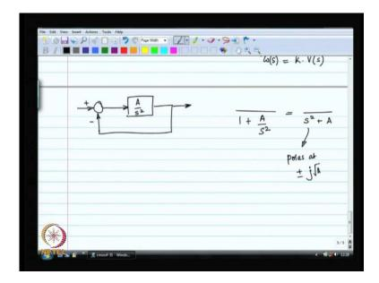
If this is your system then the denominator will have 1 plus A by S square, which means that the denominator contains this and this has two poles on the j omega axis, where are the poles. So, this kind of system is not going to be stable. So, you cannot put two integrators in the loop just like you have got to have method over here that is why you need to open your control theory book.
