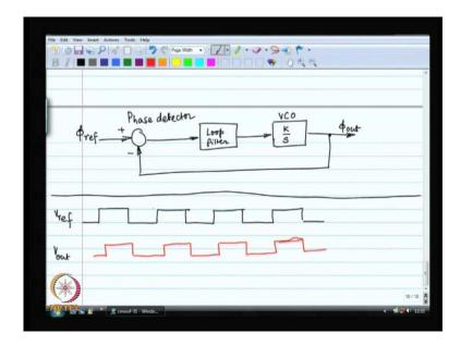
So, the general idea for our phase locked loop is this I need a phase detector then I need a loop filter, and then I have got my VCO, which is modeled as K by S. So, this is the
