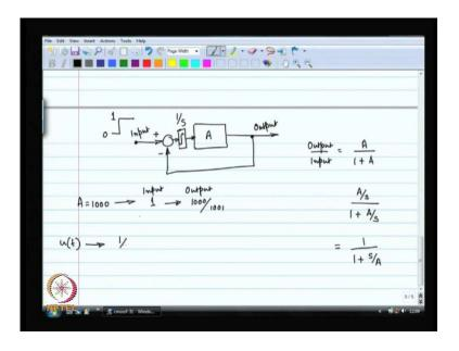
Let me give you a filler I do not want to be teaching control theory here, but let me just give you a filler of a what we are talking about suppose the input is a step going from 0 to 1 that is not the characteristics of our input, but suppose it is in any case this particular control system has again. This is the input this is my output the gain output by input equal to A by 1 plus A, open loop gain divided by 1, a loop gain divided by 1 plus 1 minus the loop gain.
