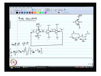
Now, another very popular oscillator is the ring oscillator it is a very popular oscillator specially in the digital world lot of ah clocks on c p u s are generated sometimes through ring oscillators. So, a ring oscillator is something very straightforward I can design a cmos inverter cmos inverter is something like this this is your cmos inverter. So, I can design a cmos inverter and I can put an odd number of these inverters in cascade odd
