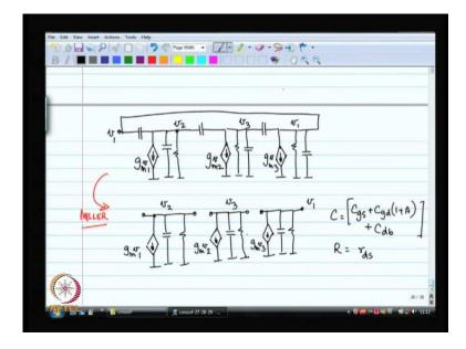
You can simplify this to this ((no audio 26:26 to 27:03)) right now these gate to drain capacitor pose some kind of problem because they are between 2 terminals and not respective to ground typically you can break this you can conceive of breaking this using miller's approximation and if I break the gate to drain capacitance using miller's approximation then it breaks up into a times where a is the gain of each stage a times c g d on 1 side and c g d on the other side.
