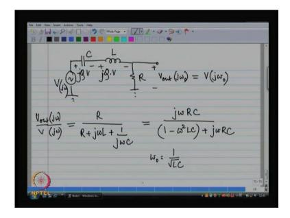
It is easy to now look at series RLC circuits. The same definition of quality factor applies here; same old definitions apply. Let us apply a voltage and exchange the configuration a little bit. Let us apply a voltage. Last time we applied a current; now, let us apply a voltage. And, we are going to measure the voltage that I developed across the resistor. So, this is a resistive divider. And, this is what we have got.
