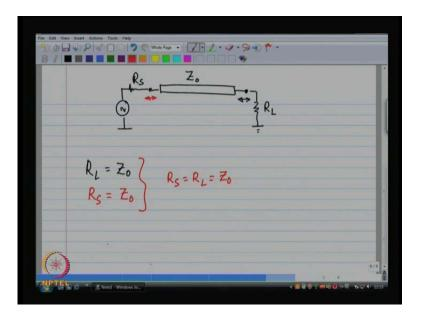
And, we concluded as follows that, if I have a source; then, to avoid reflections, I would like to have R L to be equal to Z naught. To avoid reflections at this interface, I would like R L to be equal to Z naught. And, to avoid reflections at this interface, I would like R S to be equal to Z naught; which eventually means that R S should be equal to R L should be equal to Z naught. Now, this is just a coincidence. It also naturally gives us maximum power transfer.
