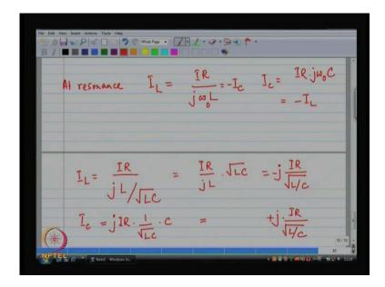
Now, let us see if that works out. Omega 0 is 1 by square root of LC. So, this is the current through the inductor. And, the current through the capacitor is going to be the same with a plus sign hopefully; wonderful. So, they match up; the current through the inductor is the negative of the current through the capacitor. Now, what you observe is a factor. So, the current through the inductor...
