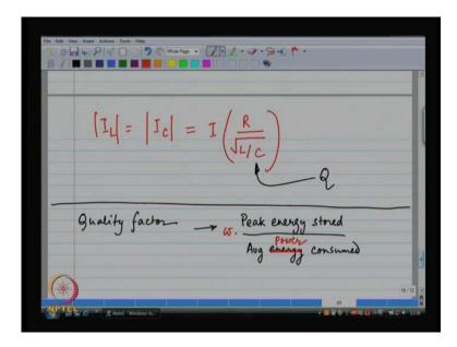
Let us look at the modulus of the current through the inductor, which is equal to the modulus of the current through the capacitor. And, that is going to be I times R by square
