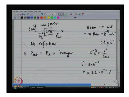
When we are talking about an RF system, we have an antenna and then we have an LNA – a low noise amplifier. We want maximum amount of power possible to be received on the low noise amplifier; why? Why do I want maximum power on the signal to be received on to the LNA. It so happens that, maximum power received on the LNA also means that, there are no reflections; that is a coincidence; that is a coincidence. Next important thing is that, the LNA has a finite amount of power gain.
