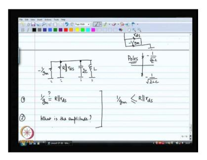
And if you re draw your thing than this is what you have got alright now it is easy to see that when minus 1 by g m is exactly equal to R parallel R d s all your left with are the inductor and the capacitor the negative and the positive [re/resistors] when they are in parallel with each other they nullify each other right in this passion this is how they nullified each other it is almost like there is an infinite resistor in chant which is nothing nothing in chant right.
