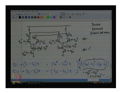
This is our double balanced gillbert cell mixer and at the end of the previous class we were struggling to figure out how we can interchange the RF and the LO terminals right this is what we were struggling to figure out at the end of the previous lecture. So, will finish with that and then we are going to talk about mixer non idealities what are the different problems with mixers how they are going to effect the radio architecture and. So, on and. So, forth all right.
