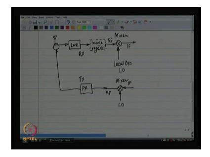
Welcome to CMOS RF integrated circuits today is a lecture 25 we are starting a new module today and this is module about mixers or multipliers. So, typically in a receiver the mixer is the second block or sometimes the third block. So, a typical receiver looks like this.
