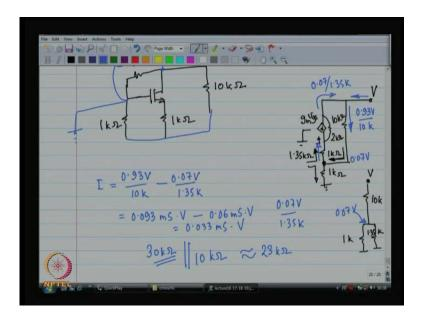
So, all these calculations you have got to do carefully. Now, C g s is 300 femtofarads, I have got 350 ohms over there. So, I should be getting something like 350 times 200. So, about 70 pico seconds, alright. And, lastly I am left with C g d; C gate to drain now, gate to drain is also going to be similar. And, for this you are going to apply your voltage over
