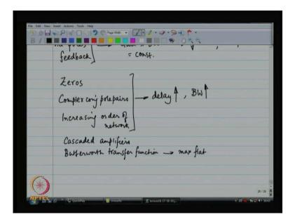
Gain bandwidth product; gain goes down, bandwidth goes up. This is really when I have got all poles, when I have got feedback around the system etcetera. The other strategy that we have got is by inserting zeros, strategically inserting zeros by using complex conjugate pole pairs by increasing the order of the network. All of these cost me in terms of delay; delay is something which I can tolerate. If I reduce the gain my system becomes less useful, if I increase the delay then there is no harm.
