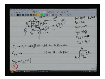
And, to do to work out the bandwidth what we have to do is we have to imply the method of open circuit time constants; I did not even consider a load R L. You basically have to put R L in shunt with whatever output resistance you have got or what you can do is you can split the gain that you have got over your R out and your RL. And, you can find out the net gain; that is also fine.
