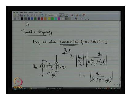
Now, the most important metric you may or may not have heard of this metric is the f T; f T is the frequency the transition frequency. Now, the definition of the transition frequency is that it is the frequency at which the current game of the mosfet is 1. Now, we have something serious over here; what on earth is current game, what do you mean, what are we talking about?
