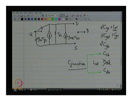
These are all the different possible capacitors C g s get the source; C get to drain, C get to body, C source to body, C drain to body and C source to drain right; of this we were proceeding one by one we evaluated C get the source and get to drain capacitances right. This 2 we evaluated; in addition to what we had evaluated there will also be a small component called the overlap.
