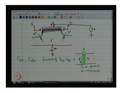
Now, really the drain and the source; these 2 are made out of n plus type of material; especially when I am talking about and n mass. And, the body is made out of p negative type of material when I am talking about the n mass; for the p mass it is exactly the opposite. We are discussing the n mass for generality, p mass you can similarly discuss identical effects will happen; for the p mass you have to remember to connect the body to the most positive voltage in your circuit.
