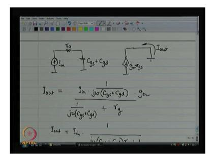
So, this is going to be the real expression which means that I in I out by I in that is your current game; I made a mistake looks like its correct I in no this is correct; I have got to have made a mistake alright that is my corrected version. In fact, which accounts for the presence of the gate resistance. Now, when that is my I out then things will slightly change over here in my previous computation, alright.
