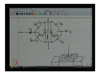
Our model for the mosfet looks like this I have got 4 terminals; gate, source, drain and body. And, between drain and source there is voltage controlled current source; this is the fundamental mosfet; to account for channel link modulation this is going to be a large resistor RDS between drain and source; between gate and source I have got a capacitance which is the sum of overlap which is intrinsic and CGS which can be changed with the biased voltages.
