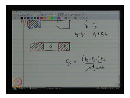
So, C junction source is going to be A S plus P S times h times epsilon of silicon divided by d of the junction; d of the junction is of course function of the source to body voltage; its source to body voltage is if its if the junction is more forward biased this d junction is going to become smaller. If the junction is more reversed biased d junction is going to become larger; that is basically the idea right; same formula applies for both source to body and drain to body capacitance.
