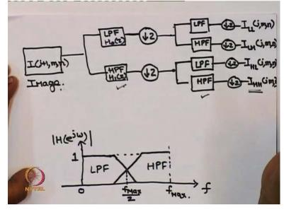
Since we have done subsampling by a factor of 2 both along the rows and along the columns, it means that in effect, we have done so sampling by a factor of 4.
