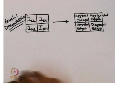
Pictorially, this can be represented as, this is our output that we have got as ILL. this is the subband where our output ILH will occur is a subband where the output IHL will occur, this is the subband that the output IHH will occur.
