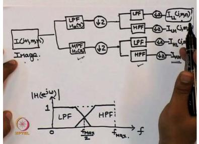
So if we perform the same operation as we have done for level 1 decomposition over here and take the output that we have obtained as ILL JMN and now consider this output as an input over here and perform the same operation that we have carried before we will get level 2 decomposition.
