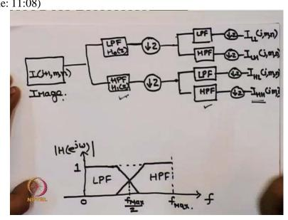
Now, it is important to observe here that the outputs subimages or at one resolution less than the image that we have started with. That is, we have in effect larger resolution by a factor of 2 along the rows of the image and also along the columns of the image.
