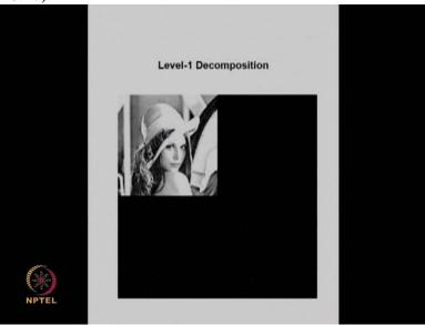
If we will do simulation of such a thing using any software like Matlab, what we will obtain is a figure like this. So this was our original image which is lena and its size is 512 x 512 and after performing the same operation as explained before, we have decomposed this original image into 4 subbands.
