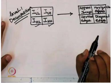
Therefore each of these subbands that is LL subband, LH subband, HL subband and HH subband contains only  $1/4^{\text{th}}$  of the total number of samples in our image originally. Now, in principle any one of these sub bands or all of these subbands can be analysed or partitioned further.
