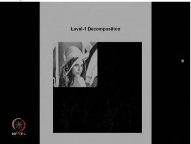
But it can be seen from the simulation here that as maximum energy or maximum information content is there in the LL subband so we would like to decomposed this band further.
