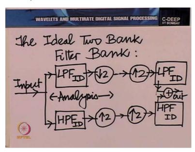
The input sequence here being fed to LPF ID ideal here, HPF ideal there, downsampled by2 subsequently, this is the analysis portion, followed by upsampled by2, again lowpass filter ideal here, high pass filter ideal here and the outputs from this are to be added to produce the overall output.
