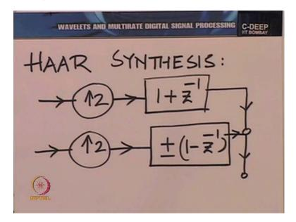
We had also derived the structure of the synthesis filter bank and interestingly we saw the structure was very similar, in fact it looked almost like a mirror image here. Except for the fact that you had an upsampler instead of a downsampler followed by the 2 filters once again.
