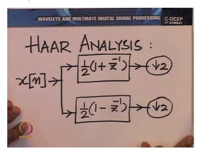
You will recall that on the analysis side we had a structure like this, we had the sequence, let us call it X of N corresponding to this the function in V 1. Essentially it was subjected to the action of 2 filters, filter of the form half 1 + Z inverse and other one of the form half 1 - Z inverse, followed by a downsampling by 2.
